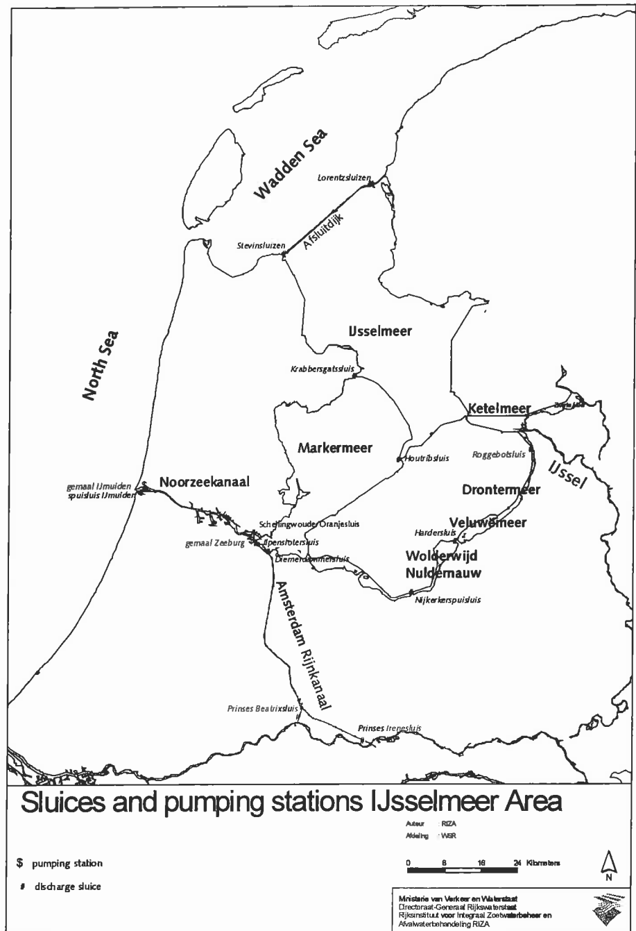
Figure 12.1 IJsselmeer area with discharge sluices and pumping station that discharge water to the area
