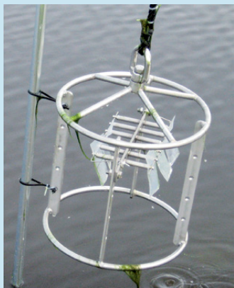
Sampling device with silicone rubber passive samplers
