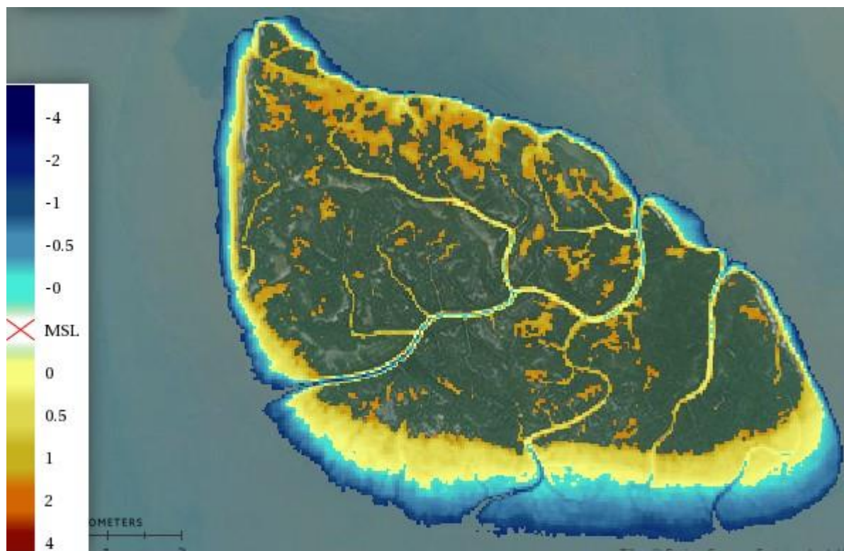
Figure 2.4. Google Earth Engine Derived intertidal Elevation dataset near the Sunderbans in Bangladesh (derived from the NASA/USGS Landsat and EU/ESA/Copernicus Sentinel 2 earth observation collections combined with CNES-AVISO+ Global tide - FES2012 tidal simulations).
