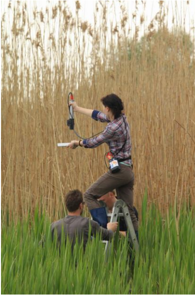
Figure 3.3. Vegetation measurements of the reflectance of reed beds in the Romanian field site.
