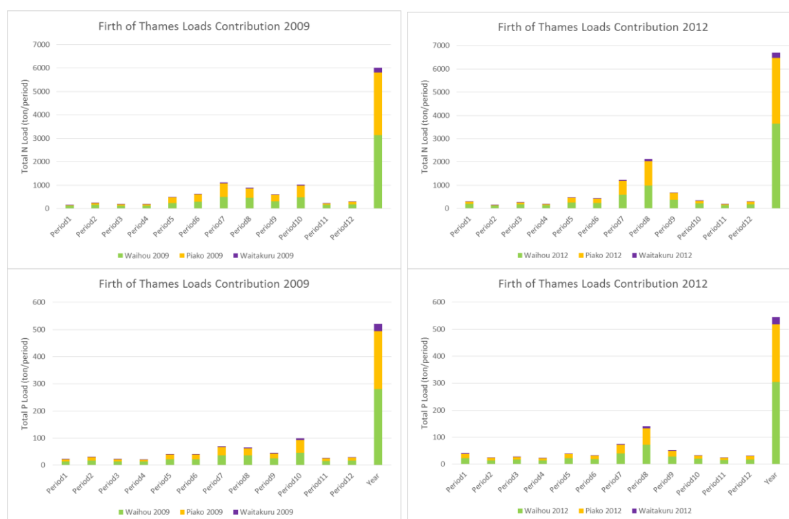
Figure 5.20 Total nitrogen and total phosphorus load contribution (top – bottom) according to the Hauraki Plains Model to the Firth of Thames by the Waihou, Piako and Waitakuru in the validation years 2009 and 2012 (left-right).
