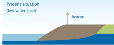
Present situation (low water level) Groyne lowering Waal River ( \pm 1 m) will be applied over a distance of approx. 60 km between Gorinchem and Nijmegen.
