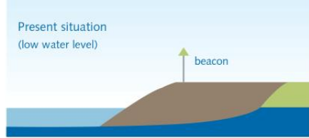
Present situation (low water level) Groyne lowering Waal River ( \pm 1 m) will be applied over a distance of approx. 60 km between Gorinchem and Nijmegen.
