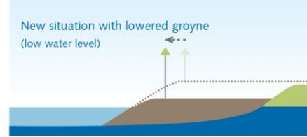
New situation with lowered groyne (low water level) Shipping beacons are on the groynes. These will be moved and extended.
