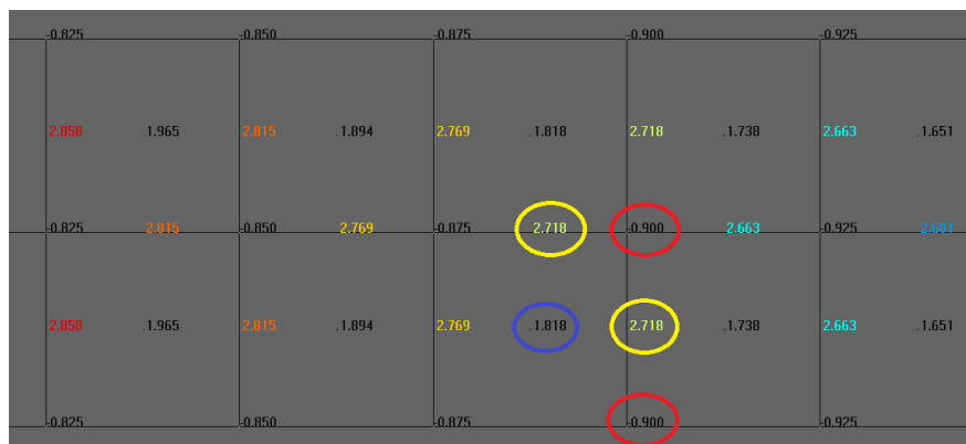
Figure 3.5: Selected part of one of the computational grids, revealing outcomes at specific locations. The water depth at a flowlink is highlighted by a yellow circle, the water level at a flownode by a blue circle and the bed level at a netnode by a red circle.
