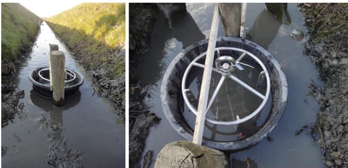
Figure 2.5 Installation of the samplers in the ditches
