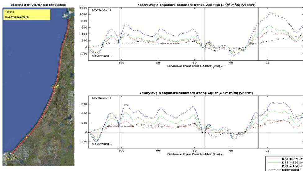
Figure 2: Computed sediment transport for 3 sediment diameters ( $D_{50}=150, 200$  and  $300 \mu\text{m}$ ) and two sediment transport formulae (Top: Van Rijn, 2004, Bottom: Bijker, 1977) (Deltares, 2010)
