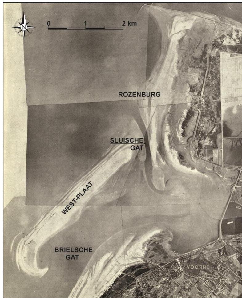
Fig. 7. Aerial photograph of the mouth of the Brielse Maas and the shoreline of the island of Rozenburg in 1961. The channels Brielsche Gat and Sluische Gat in the ebb-tidal delta have rotated to a more or less north-south orientation. The shoal Westplaat has grown in surface area, has migrated shorewards and shows recurved spits at its southern tip. In front of the island of Voorne (bottom of picture), a fan-like spit complex has formed. (From: Terwindt, 1964).
