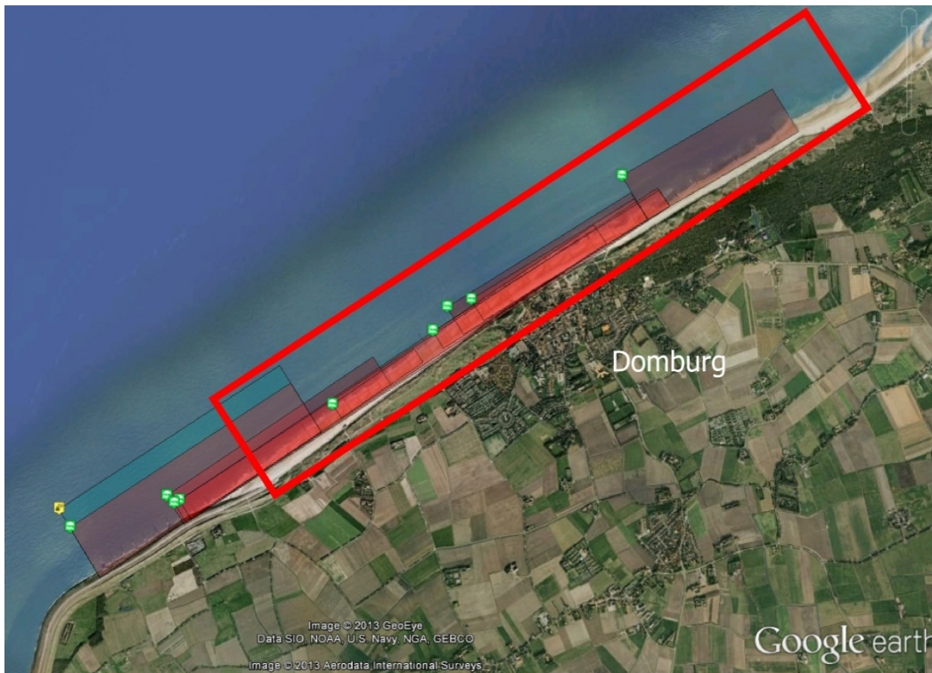
Figure 2.12 Locations of the twelve nourishments carried out in and around the model area (indicated by red box) in the period 1990–2008.
