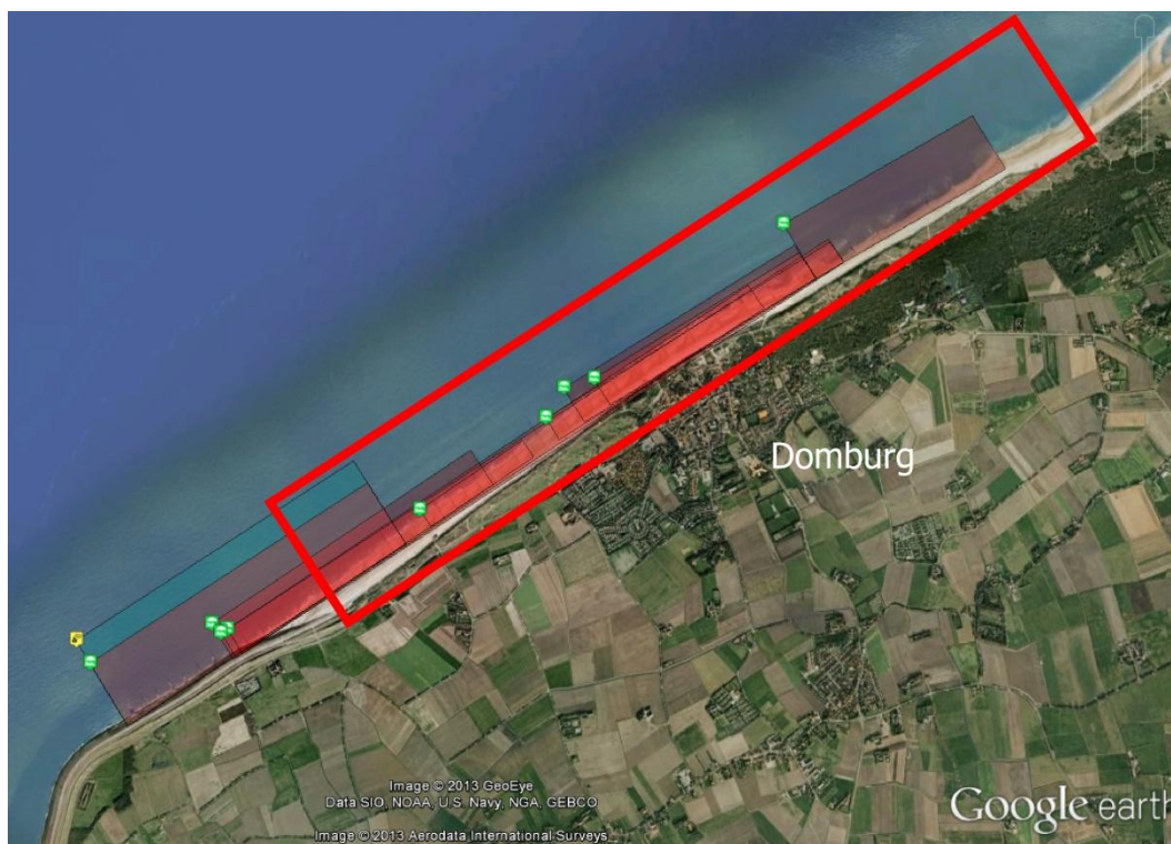
Figure 3.4 Locations of the twelve nourishments carried out in and around the model area (indicated by red box) in the period 1990–2008.
