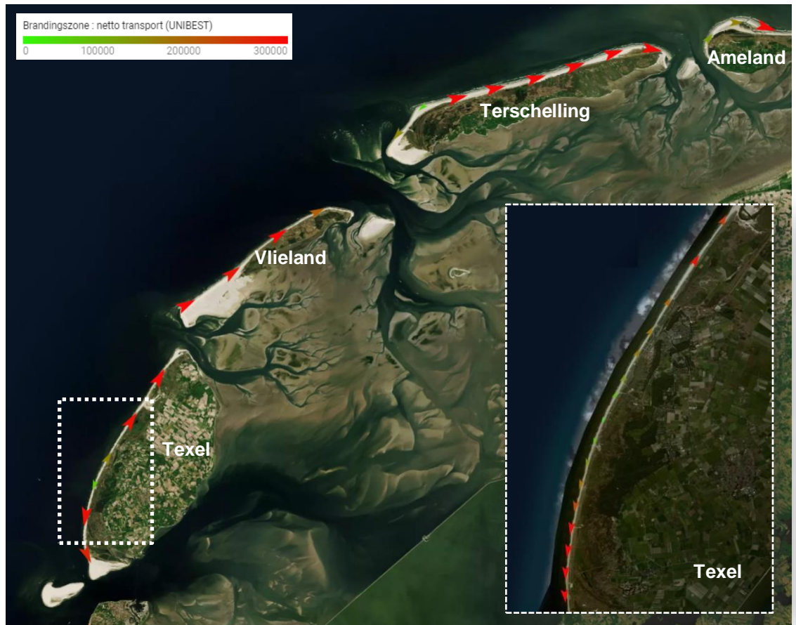
Figure 3.8 Illustrations of computed transports in the nearshore due to wave-driven currents at the Wadden coast with a detailed zoom of Texel (UNIBEST-CL+)
