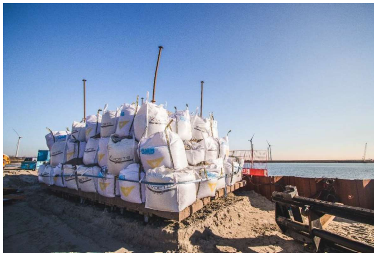
Figure 5. Arrangement of the full-scale load test in the field
