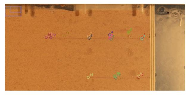
Figure 94: Manually tracked points: both transverse ribs are tracked as well as soil particles just above or below the transverse rib in order to compare the displacements.
