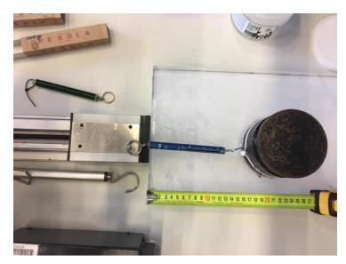
Figure 39: Spring suspension test
