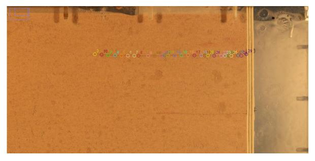
Figure 61: All tracked transverse ribs in order to compute the difference in length between the adjacent ribs and calculate the axial strain. The transverse ribs are ~5 mm apart from each other.
