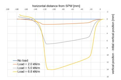
Figure 118: Deformed top geogrid-anchor at different load levels (two-geogrid configuration).
