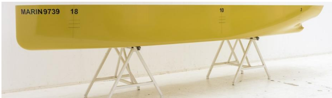
Figure 2.5 Scale model of the bulk carrier.
