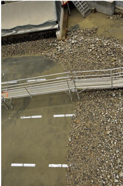
Figure A.7 Top view of damping material in the upper left corner of the Delta Basin ( X = 0 m, Y = 40 m).
