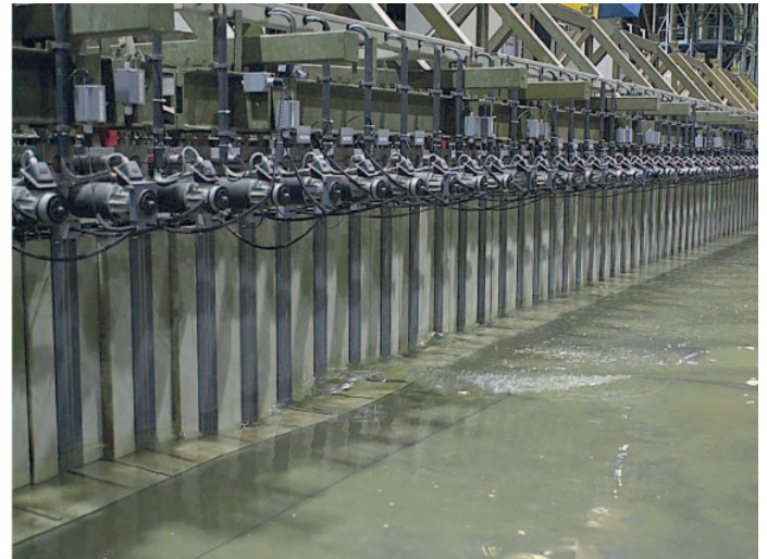
Wave generator creating a small wave
