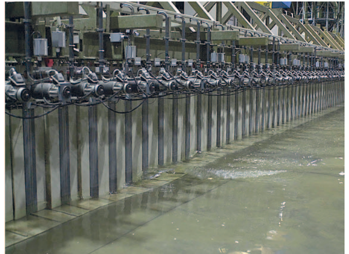
Wave generator creating a small wave
