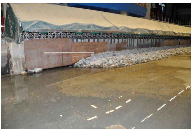
Figure A.2 Lower view of damping material along left boundary of the Delta Basin ( X = 0 m). Wooden plates are placed along the not used second wave machine.
