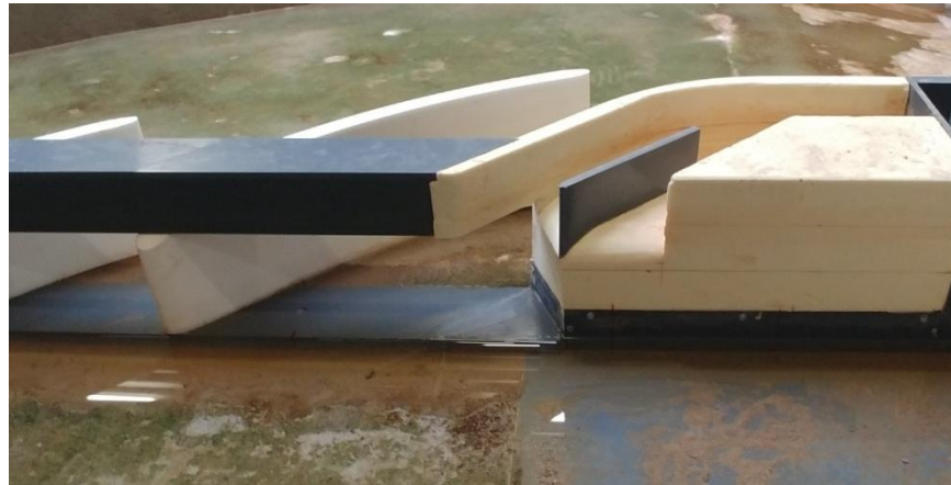
Downstream passage at IR: initial design (left) and optimised design (right)
