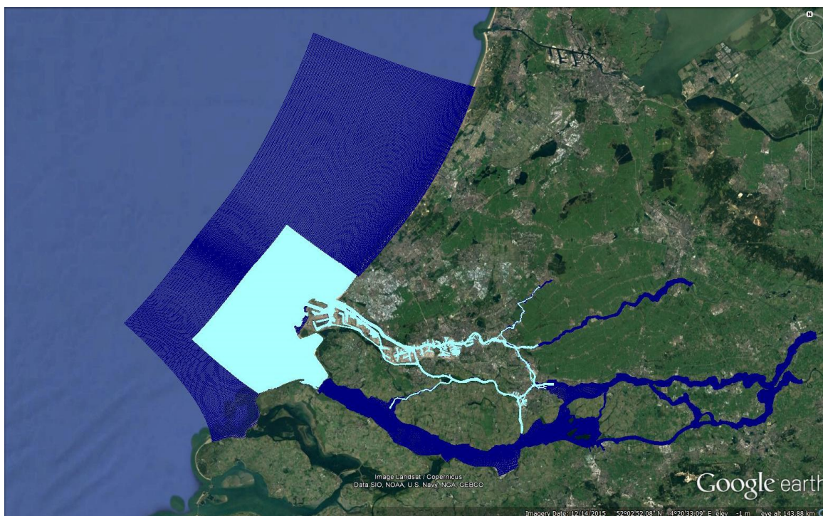
Figure 1.1 Overview of the domains from the OSR model. In dark blue the large domain (Harbour model) and in light blue the smaller domain (NSC).
