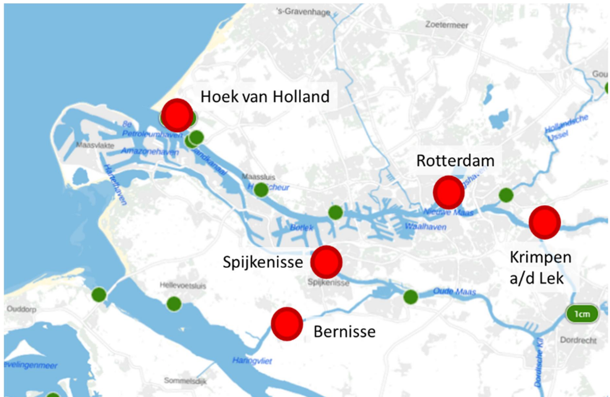
Figure A.1 Map with an overview of the RWS water level measurement stations (map taken from www.waterinfo.nl ). In red the stations evaluated in this section are given.
