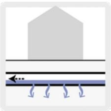
A sewage system using a perforated horizontal pipe wrapped with geotextile, drains the ground, allows water to infiltrate and transports it. Such systems are used next to paved surfaces or next to unpaved surfaces that do not offer sufficient room for infiltration ditches or where the ground has an insufficient permeability factor.
