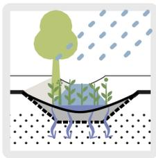
A bioswale is a ditch with vegetation, a porous bottom and below that a layer of gravel, packed in geotextile with an infiltration pipe/drainpipe. It allows rainwater storage, infiltration and transport while helping to enhance biodiversity and quality of life.
