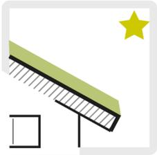
A green roof is a multi-layered roof system that is partially or entirely covered with vegetation. Extensive green roofs have a maximum depth of six (6) inches and are a layered system containing growing media, waterproofing membrane, drainage, and often irrigation components. Extensive green roofs can support groundcovers and shallow root plant material, and therefore require less structural support and reduced maintenance when compared to intensive green roofs.
