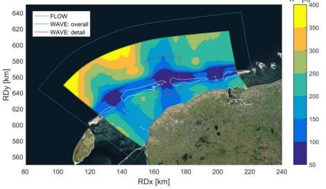
• 2D flow-wave-sediment coupled model with validated waves, water levels, flow velocities, discharges (frame locations, gorge and tidal divides)
