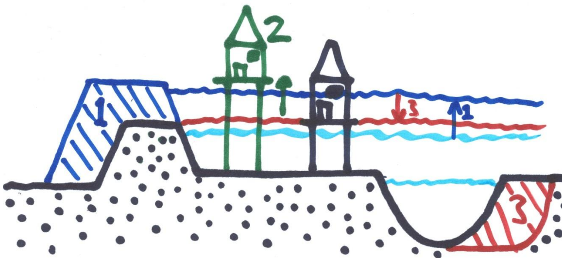
Figure 6 (to be improved) Schematic representation of three types of adaptation actions for a river flooding example. Type I increases capacity (raising dikes), Type II reduces sensitivity (raising houses, or “flood proofing”) and Type III decreases the hazard (dredging or making room for the river lowers the water level)
