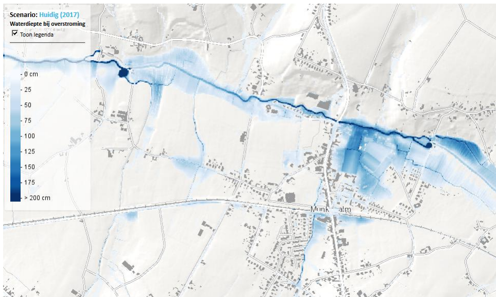
Figure 4.1 Current flood water depth around the Munkzwalm municipality during an 1:1.000 event. Source https://klimaat.vmm.be/nl/kaartapplicatie-thema-2
