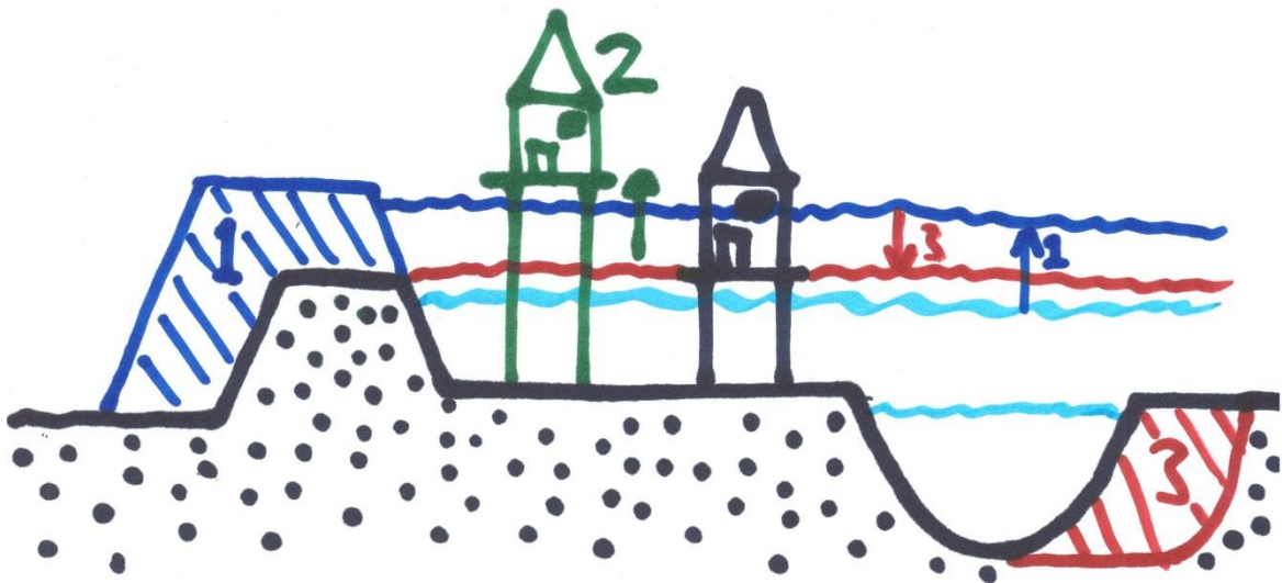
Figure 0.1 The three different types of adaptation measures, illustrated for the rise of the river flood level in embanked areas. Black lines portray the current situation. Light blue lines depict the current low and high river levels. Measure 1: increase coping capacity for increased flood water levels by raising the height and strength of the levees. Measure 2: decrease sensitivity of buildings in the flood plain by raising the building height. Measure 3: decreasing the flood level (and therefore decreasing the pressure) by widening the river bed.
