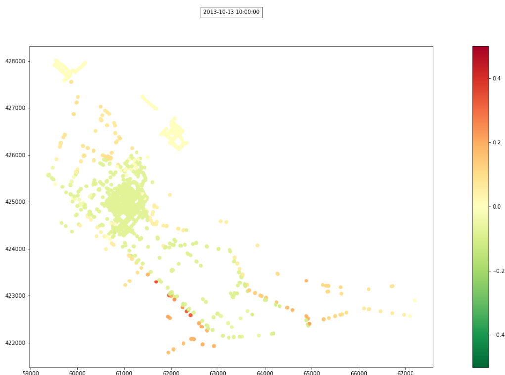
Figure 38: The difference in the calculated maximum water level between the reference model and the model with adjusted weirs at time step 13-10-2013 10:00:00
