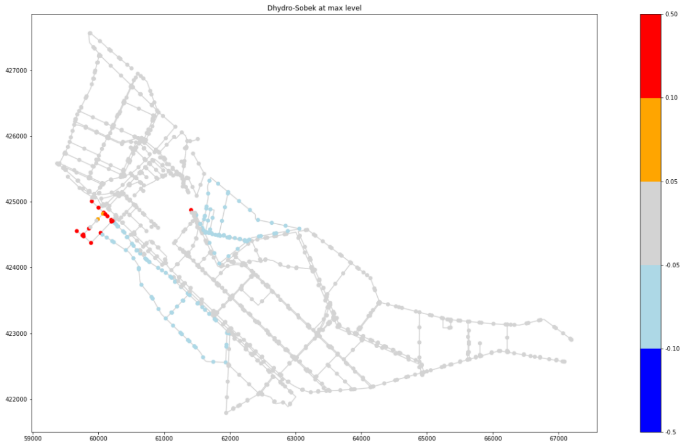
Figure 25: The difference in the calculated maximum water level between D-HYDRO and SOBEK2 for the event with 50 millimeter precipitation
