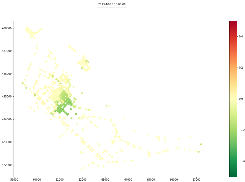
Figure 33: The difference in the calculated maximum water level between the reference model and the model with adjusted calamity weirs at time step 13-10-2013 10:00:00
