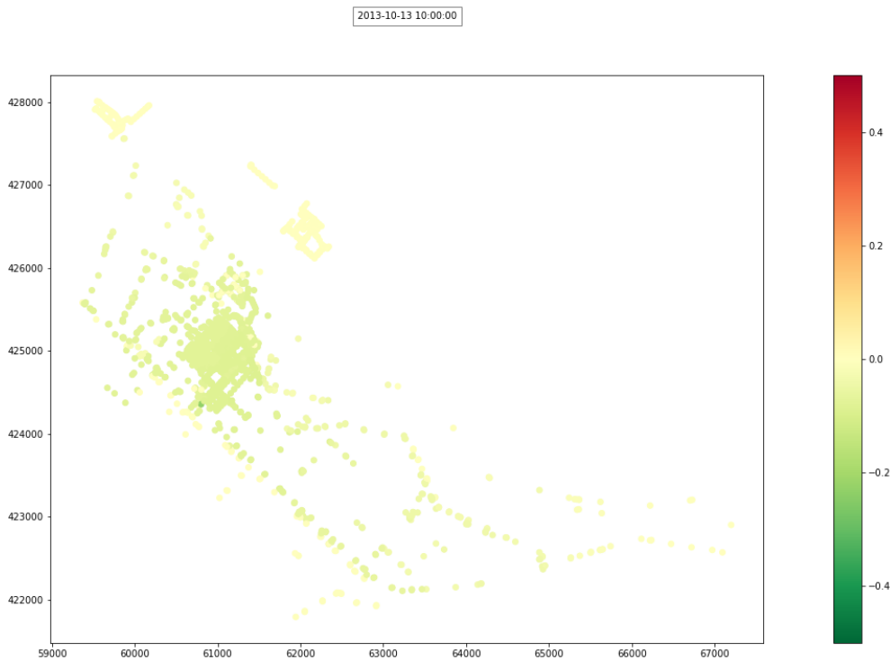
Figure 35: The difference in the calculated maximum water level between the reference model and the model with adjusted pumping capacity at time step 13-10-2013 10:00:00
