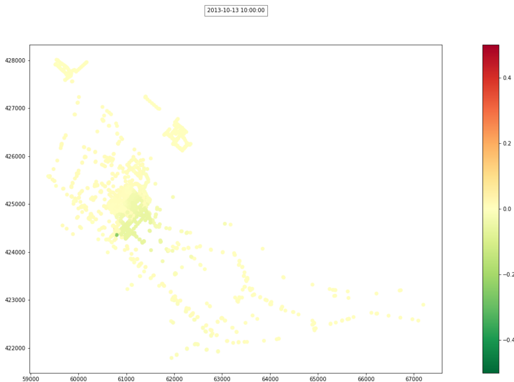
Figure 30: The difference in the calculated maximum water level between the reference model and the model with calamity weirs at time step 13-10-2013 10:00:00
