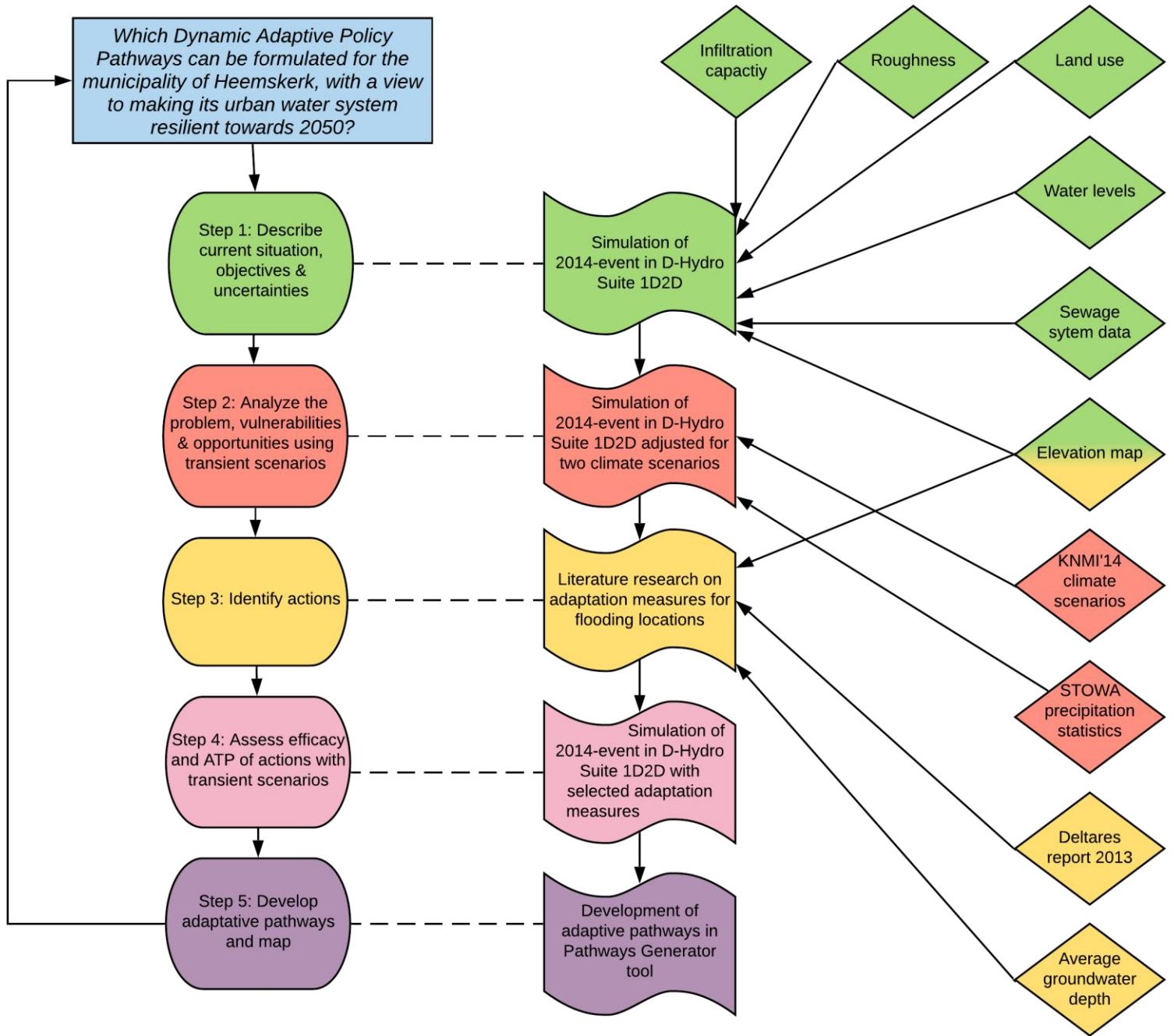
Figure 5: Setup of methodology. The round shapes show the first five steps of the DAPP approach. The flag shapes display the connected methods to the different steps. The diamond shapes show the required data. The different colors connect each step with its methodology and data.
