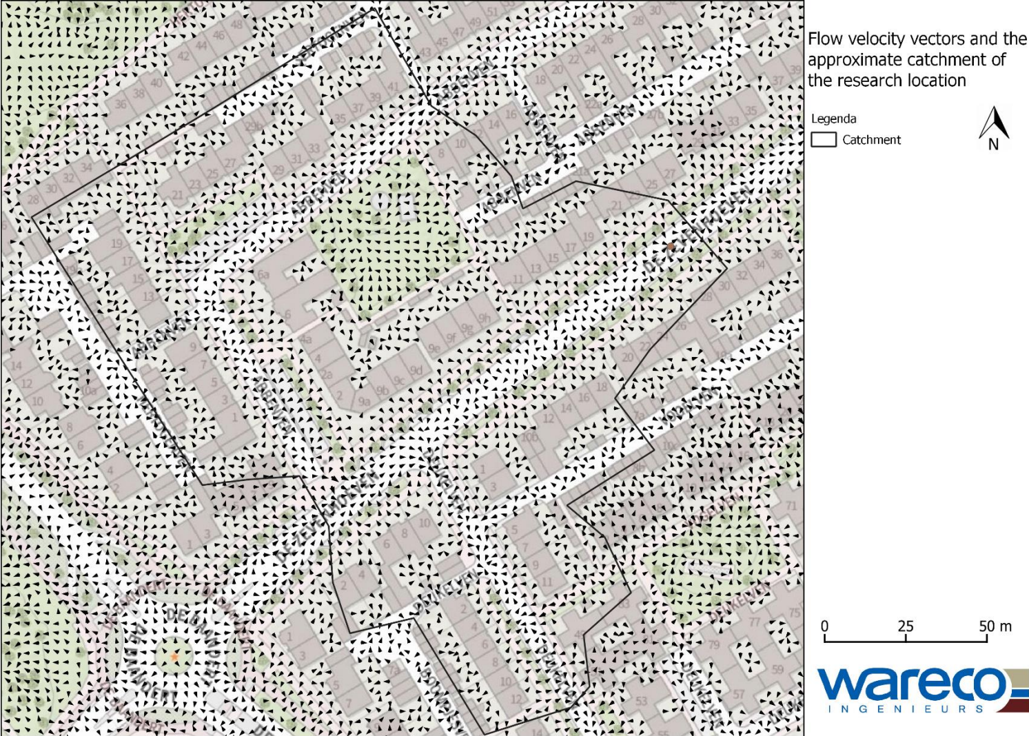
G 1: Flow velocity vectors and the derived catchment of the research location De Zevenhoeven.
