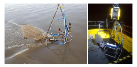
For sediment sampling a Van Veen grab, core sampler and drop core are available. In addition several instruments are available for measuring bed densities (see Section 4.2). For measuring settling velocities, HRW has a flocculation camera available (see Section 4.2), which will be used during several field campaigns. This brings the opportunity to do comparative measurements with both the settling tube and the flocculation camera.
