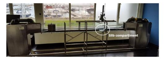
Wave-current flume, WaterProof This flume is illustrated in the figure below. It has a length of 14 m, a width of 0.5 m and a height of 0.6 m. Current velocities can be increased up to 1.0 m/s and waves can be generated as high as 0.4 m.
