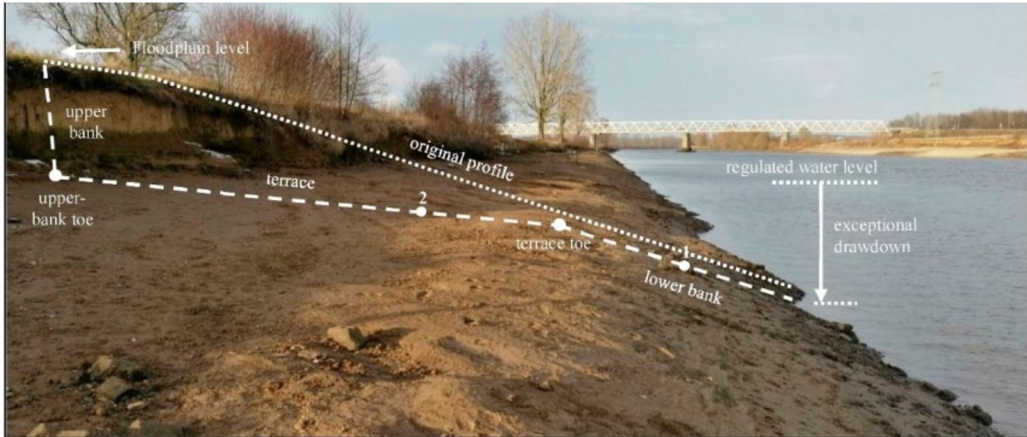
Figure A-1. Features of a bank profile shaped by ship waves along a regulated reach of the Meuse River (km 154.1), visible after a ship accident against Grave weir (source: Duró et al., 2020b).
