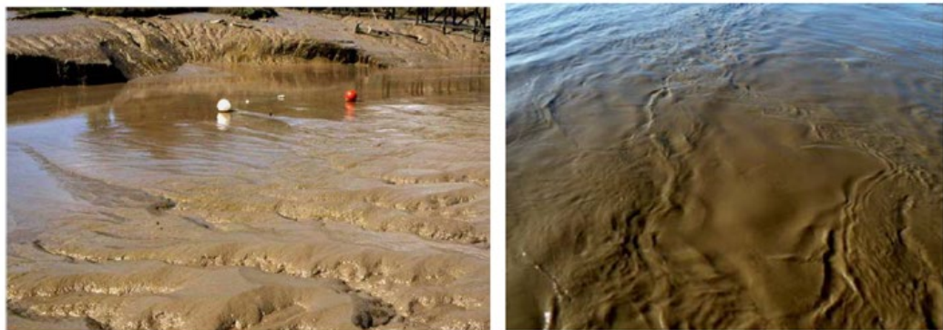
Figure 1.5 Left: stiff consolidated mud. Right: weak fluid mud (from Kirichek et. al., 2018).
