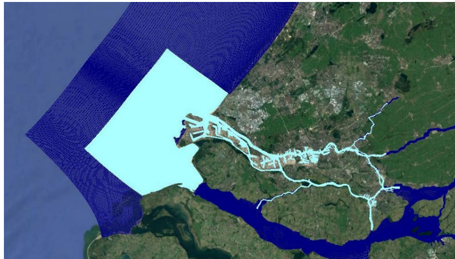
Figure 2.13 Domain of the OSR-NSC model, which was used as a basis in this model study (light blue).
