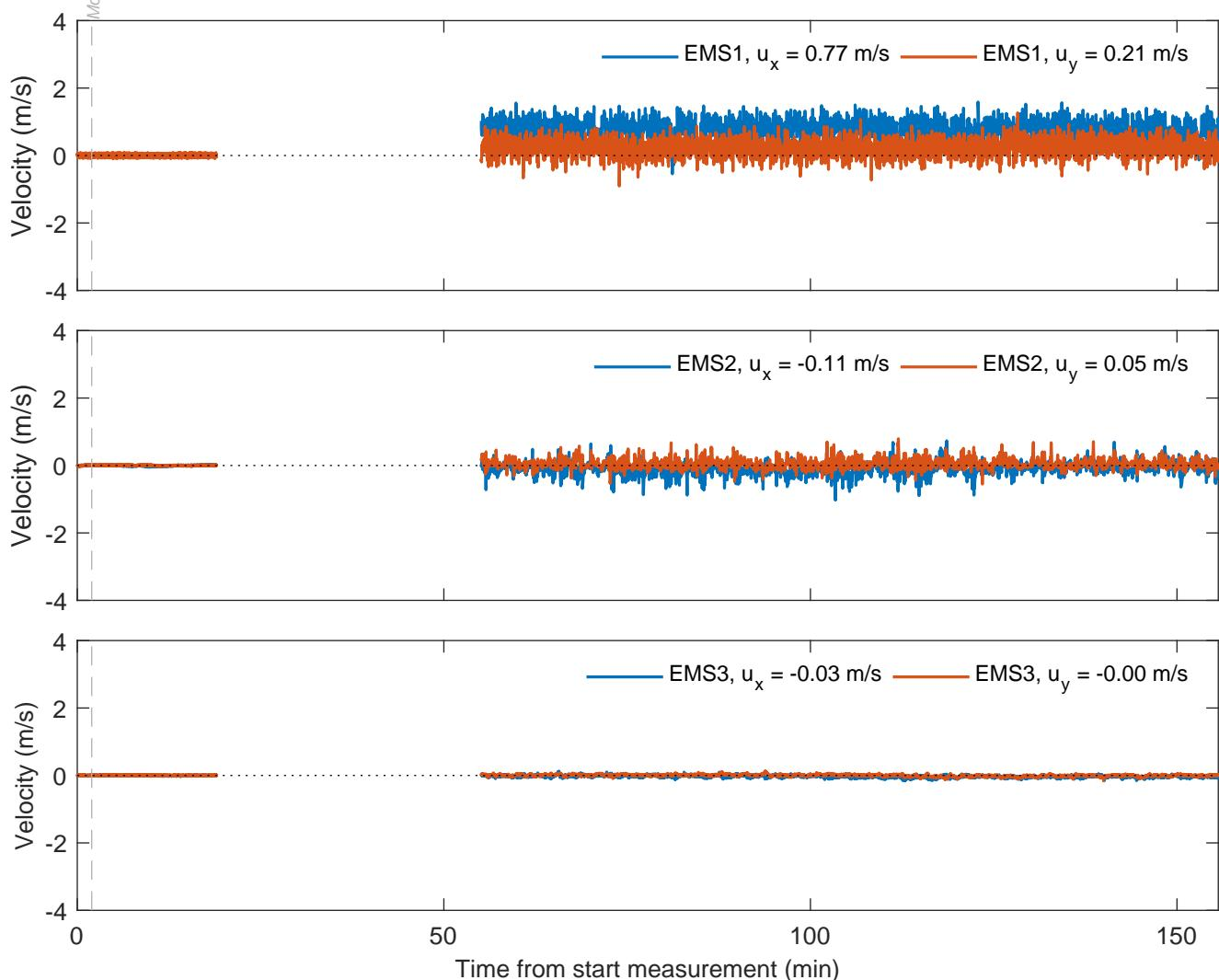
Velocities measured with EMS, x and y components
