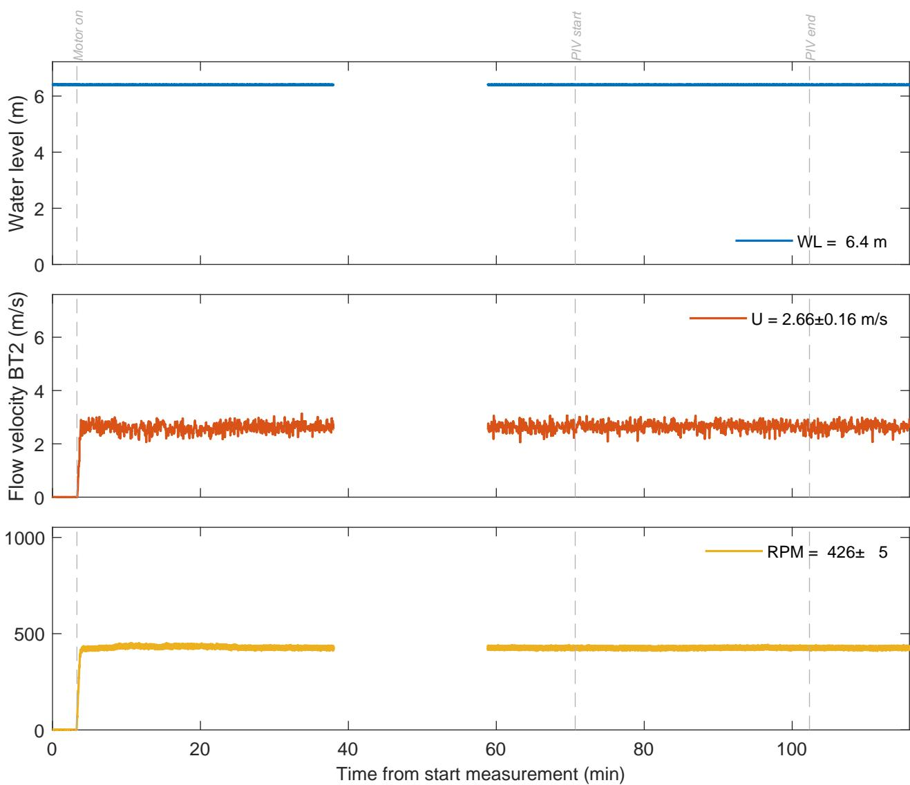
Water level, flow velocity BT2, RPM motor
