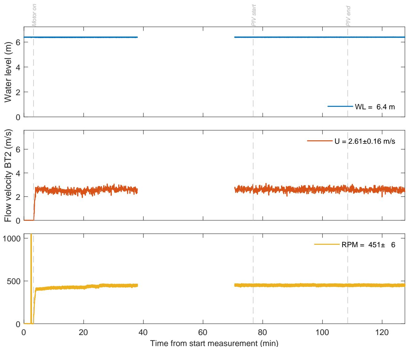
Water level, flow velocity BT2, RPM motor
