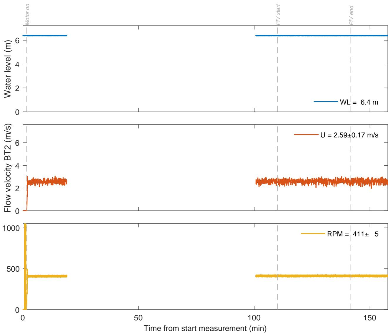
Water level, flow velocity BT2, RPM motor
