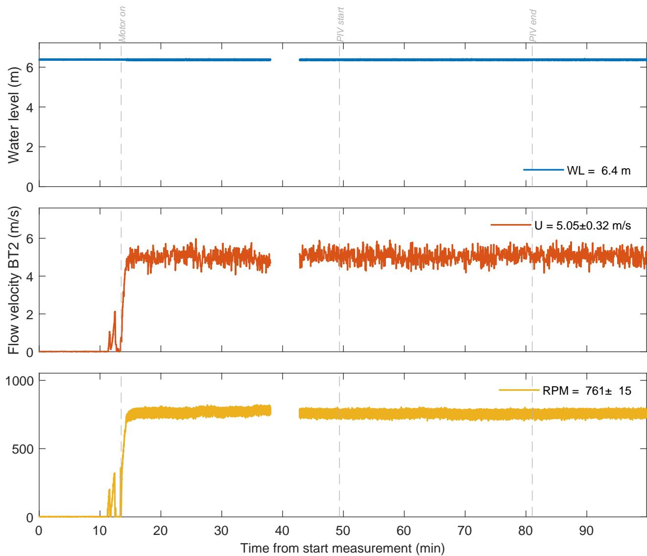
Water level, flow velocity BT2, RPM motor
