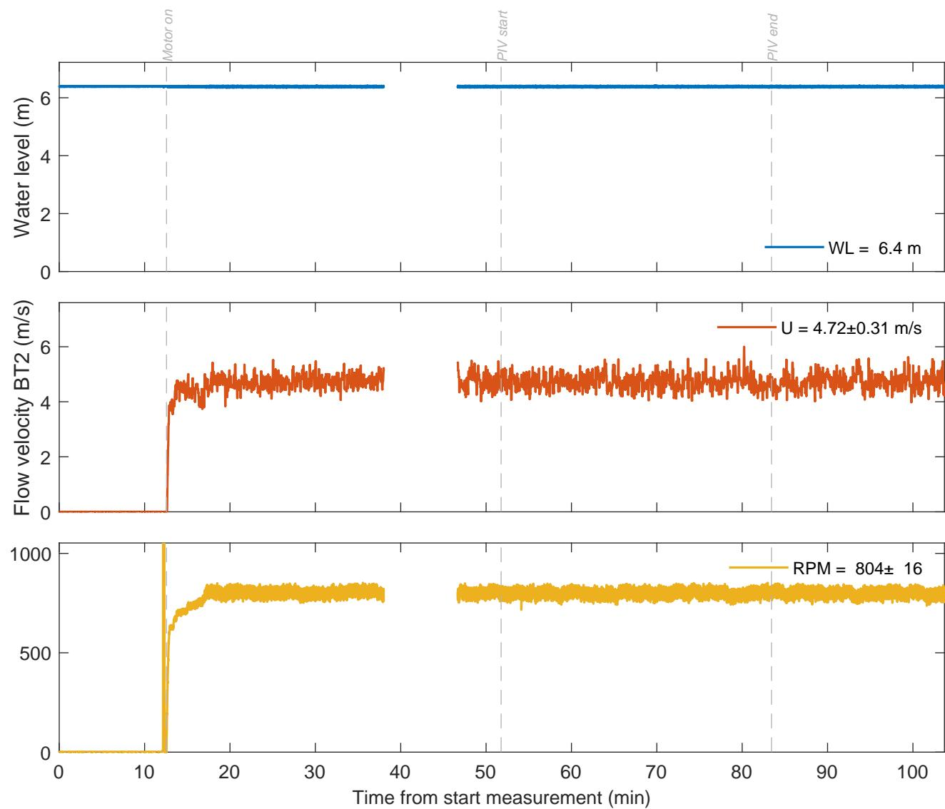
Water level, flow velocity BT2, RPM motor
