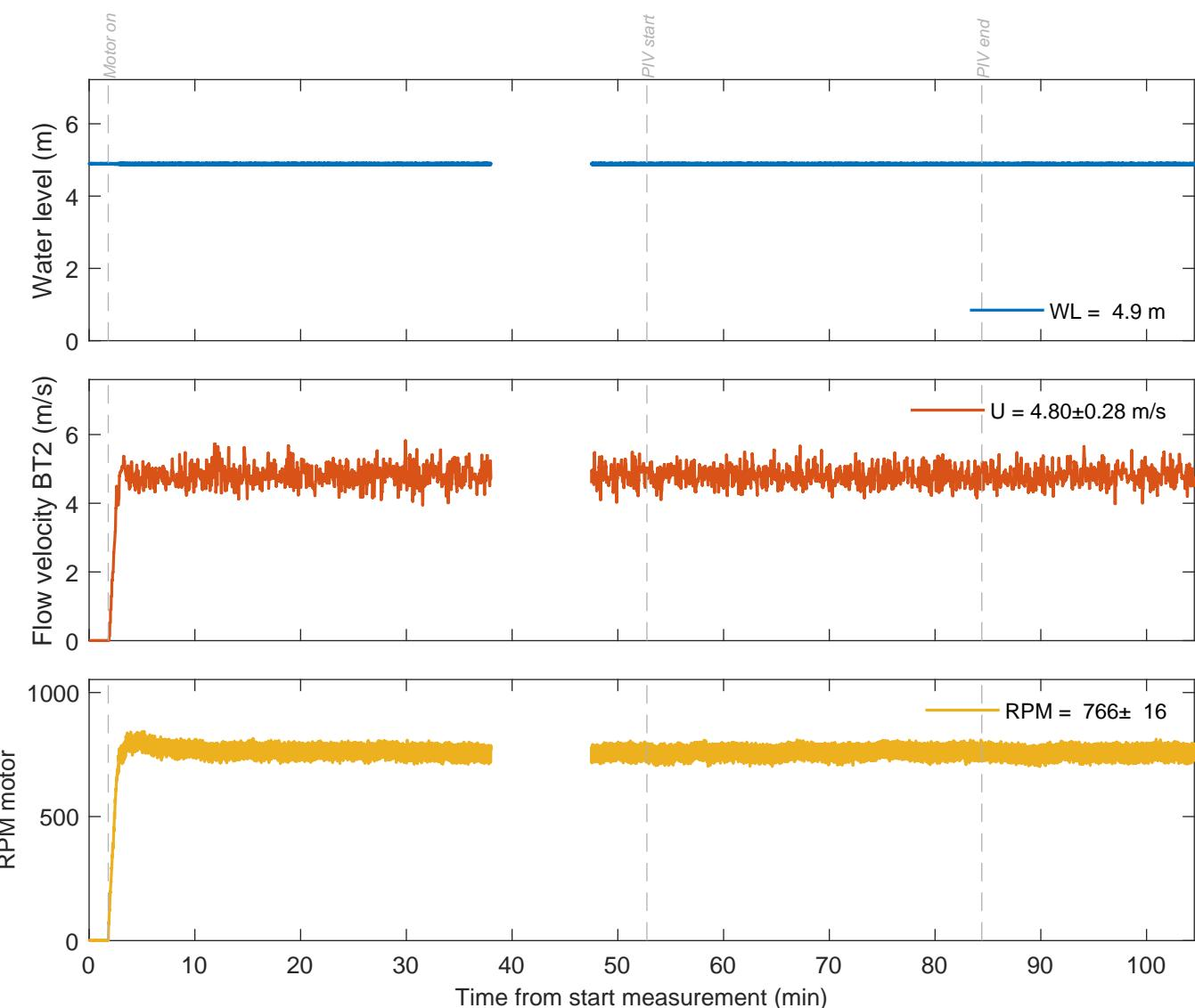
Water level, flow velocity BT2, RPM motor
