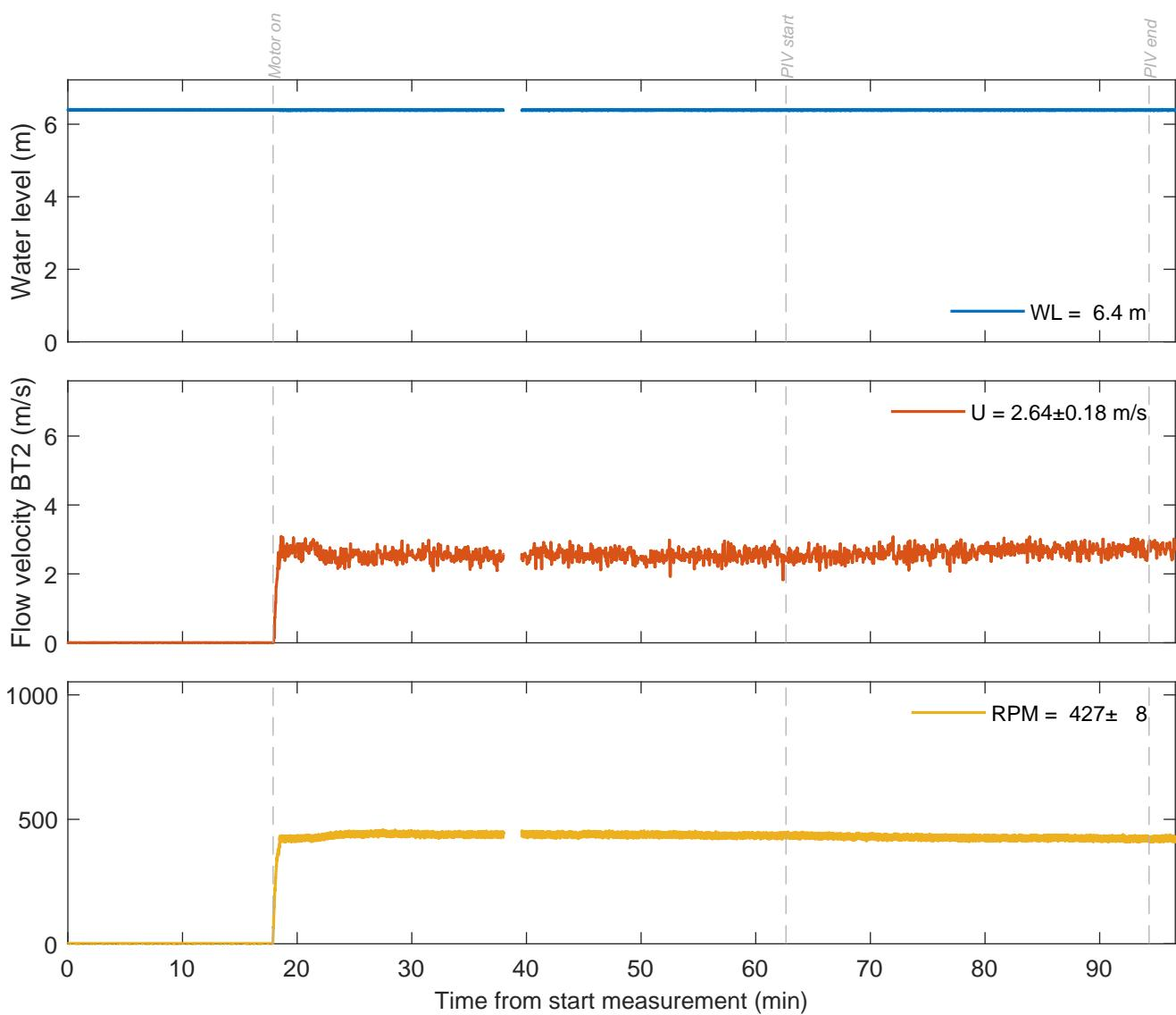
Water level, flow velocity BT2, RPM motor
