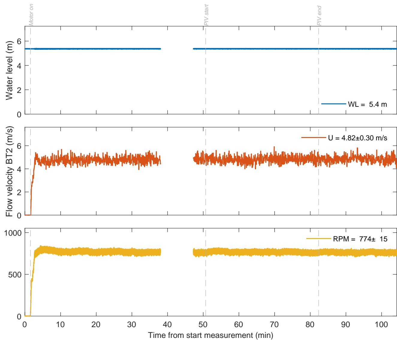
Water level, flow velocity BT2, RPM motor
