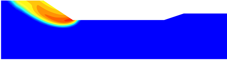
Figure 4.10 Failure mechanism for the SHANSEP MC model
