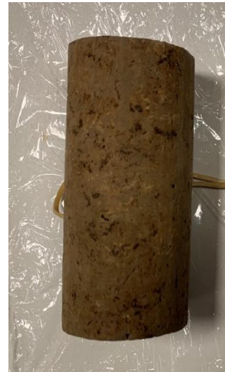
Figure 40 . Drying stage on sample T4 S2 UU-d (picture at the end of the drying stage)
