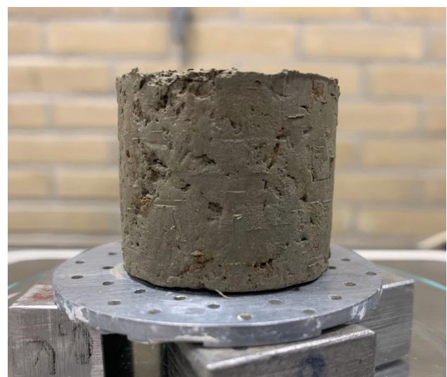
Figure 58. Results of the shrinkage test on sample T3 S4 SSC
