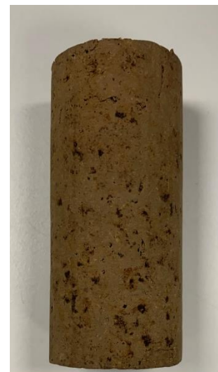
Figure 41 . Drying and wetting stage on sample T4 S3 UU-dw (picture at the end of the drying stage)
