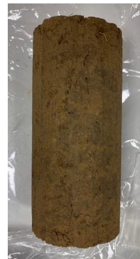
Figure 27 . Drying stage on sample T3 S1 UU-d (picture at the end of the drying stage)
