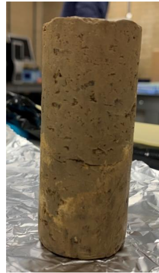
Figure 19. Drying stage on sample T7 S1 UU-d (picture at the end of the drying stage)
