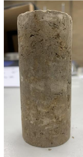
Figure 42. Drying and wetting stage on sample T5 S1 UU-dw (picture at the end of the drying stage)
