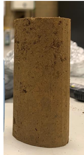
Figure 26 . Drying stage on sample T1 S1 UU-d (picture at the end of the drying stage)
