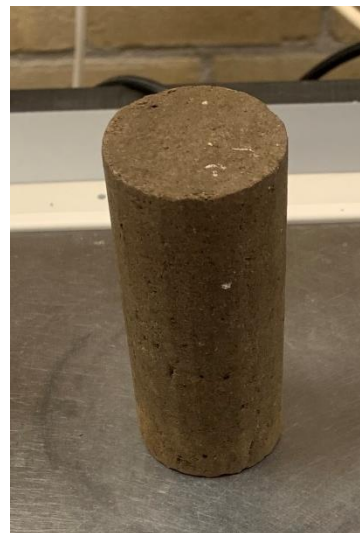
Figure 48. Drying stage on sample T2 S1 UU-d (picture at the end of the drying stage)
