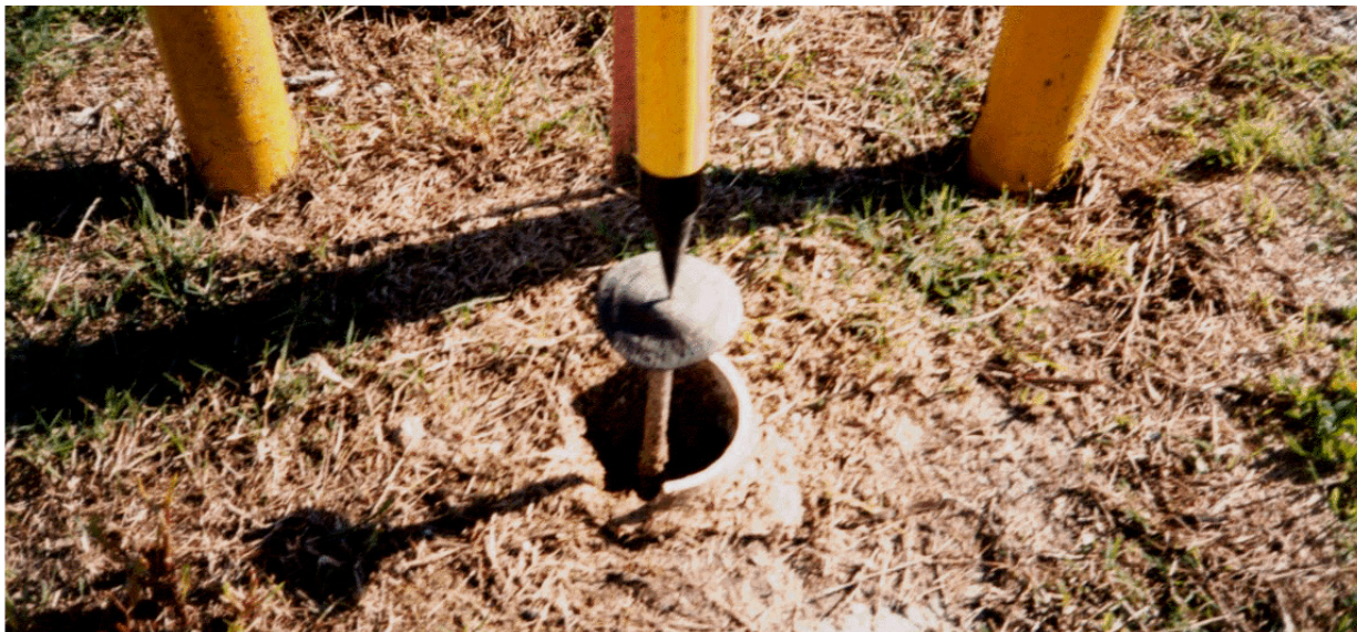
Figure 3.23 Shallow 'single-point' extensometer at Cocodrie. Subsurface and historical conditions not known. From: 2014 01 17 - Subsidence in LA-Elevations-A Moving Target LSU.pdf; by Mugnier (2014).
