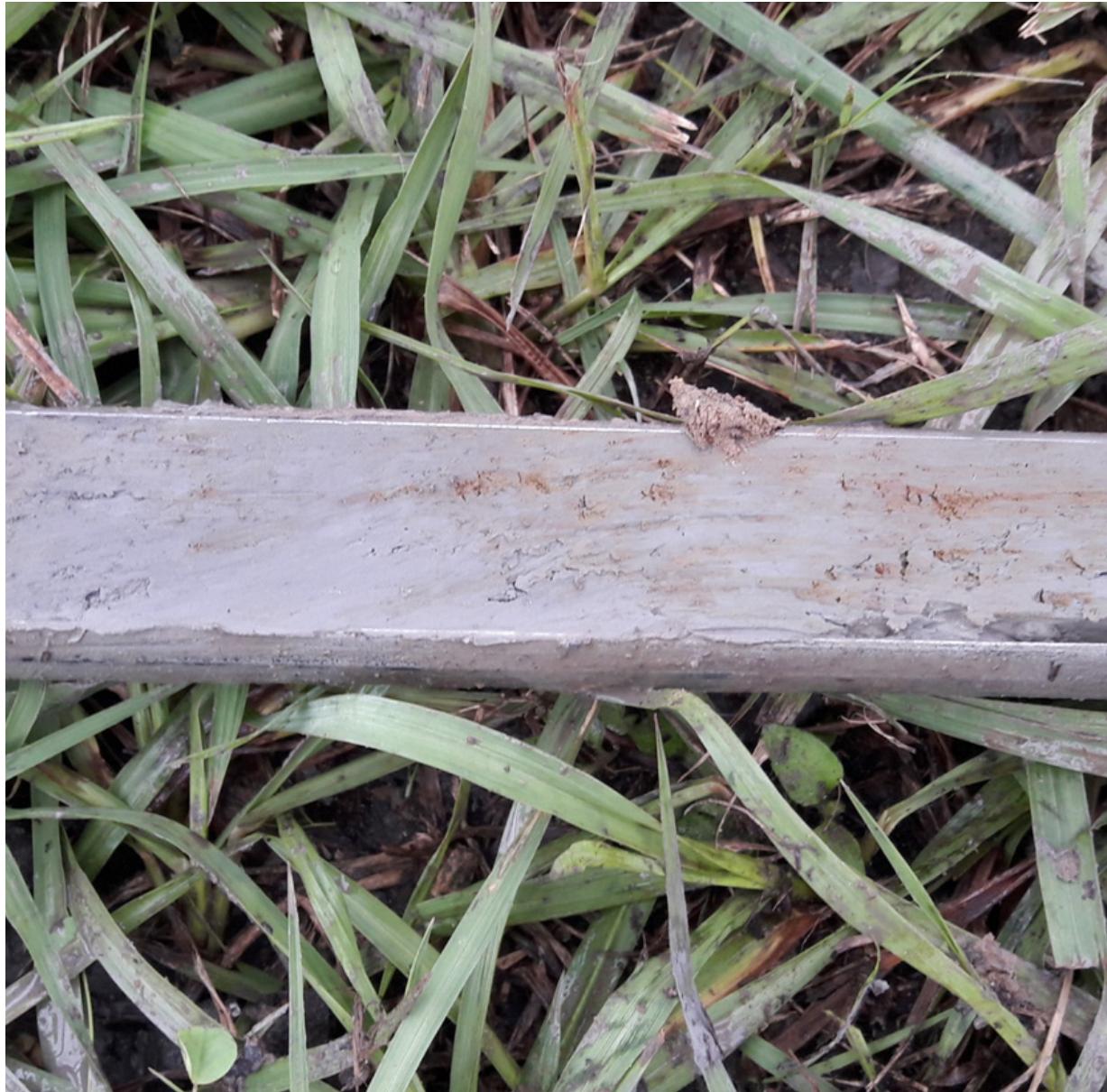
Image 2.1. Sample of oxidation in the subsoil.
