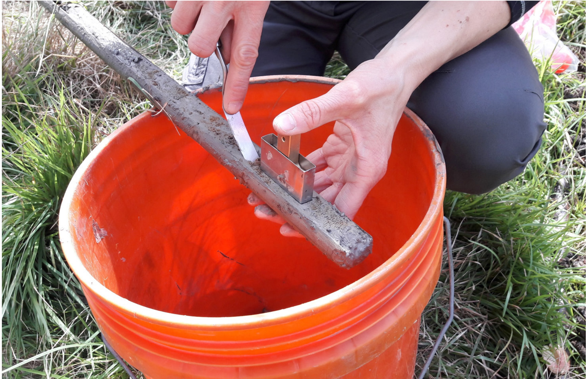
Image 2.2. Sampling an organic interval using a 1 cm x 1 cm x 5 cm sampler.
