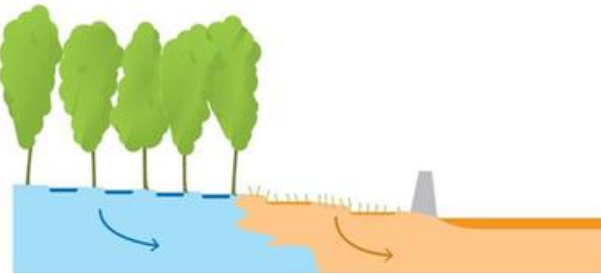
Figure 5.9 (c) Stage 3 - Civil structures and water management practices begin to transform the local ecosystem, reclaiming land by draining a section of the cypress swamp and inducing a flow reversal in the process. Now, the salty groundwater system stemming from Lake Pontchartrain now drains towards the freshwater of the cypress swamp.
