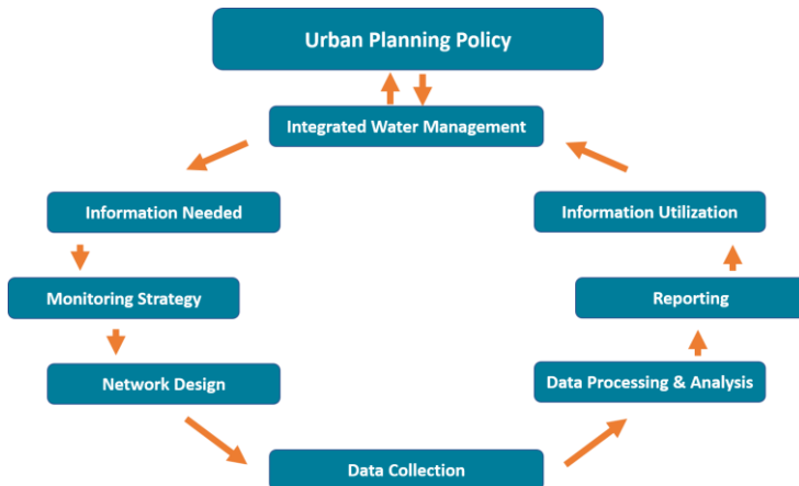
Figure 4.2 Integrated water management monitoring cycle steps and its relationship with urban planning policy decision makers.
