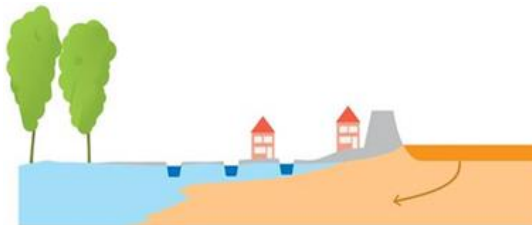
Figure 5.9 (c) Stage 3 - Civil structures and water management practices begin to transform the local ecosystem, reclaiming land by draining a section of the cypress swamp and inducing a flow reversal in the process. Now, the salty groundwater system stemming from Lake Pontchartrain now drains towards the freshwater of the cypress swamp.
