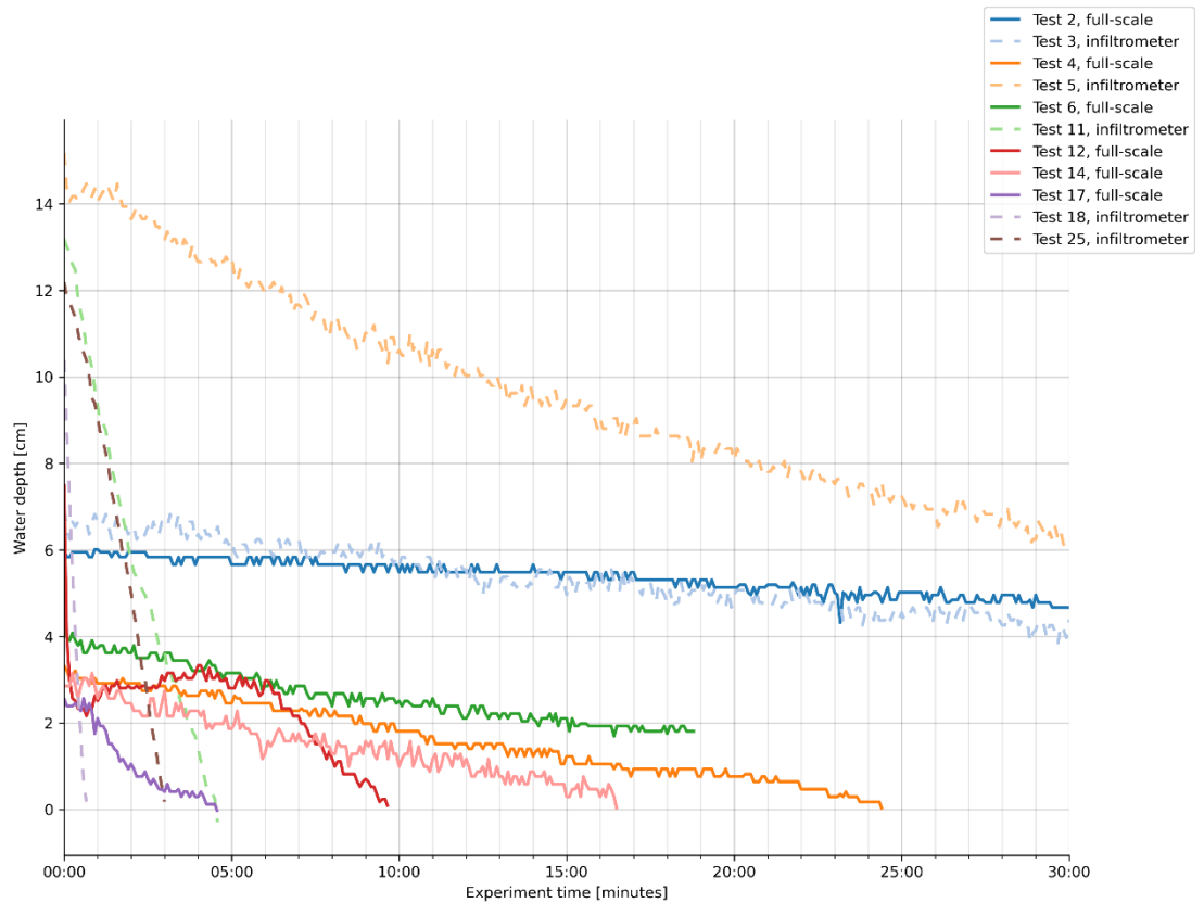
Figure 6.9: Aggregated infiltration capacity of the tested permeable pavement facilities. The number in the legend responds to the test number given in Table 6.2.
