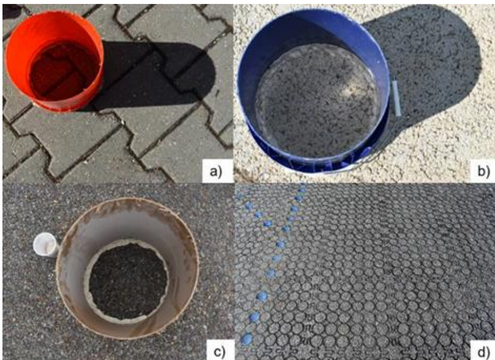
Figure 6.5: Permeable pavement variants in New Orleans during testing (a) Impermeable concrete interlocking pavers; (b) porous concrete; (c) porous asphalt; (d) plastic grid pavers.
