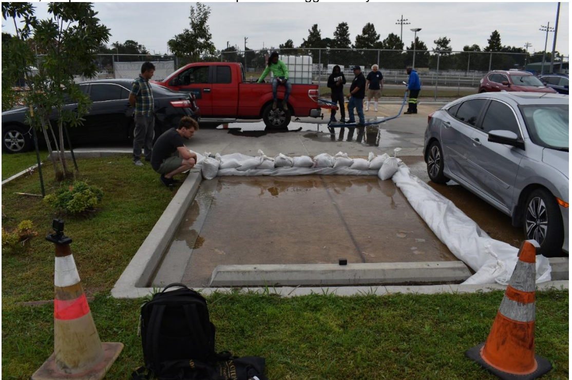
Figure 6.7: Example of a full-scale permeable pavement test (parking SWBNO)
