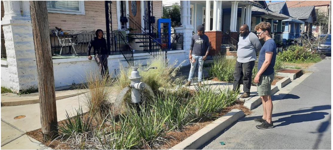
Figure 6.6: Example of rain garden test, making use of fire hydrant.
