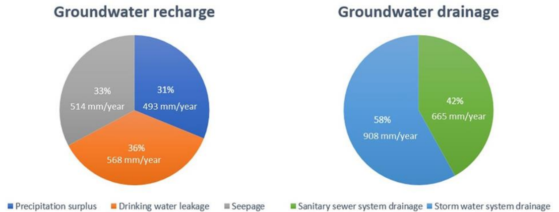
Figure 3.4: The proportions and quantities of the various fluxes in the period 2018-2020 (precipitation 1,782 mm/year and evaporation about 1,289 mm/year).
