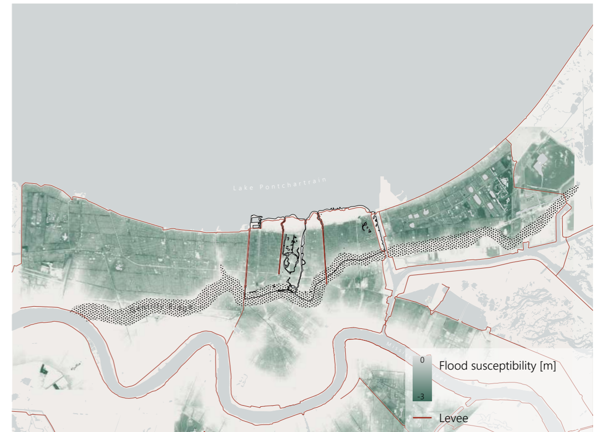
Figure 40 - Digital elevation model of New Orleans with levee system and Gentilly Ridge.
