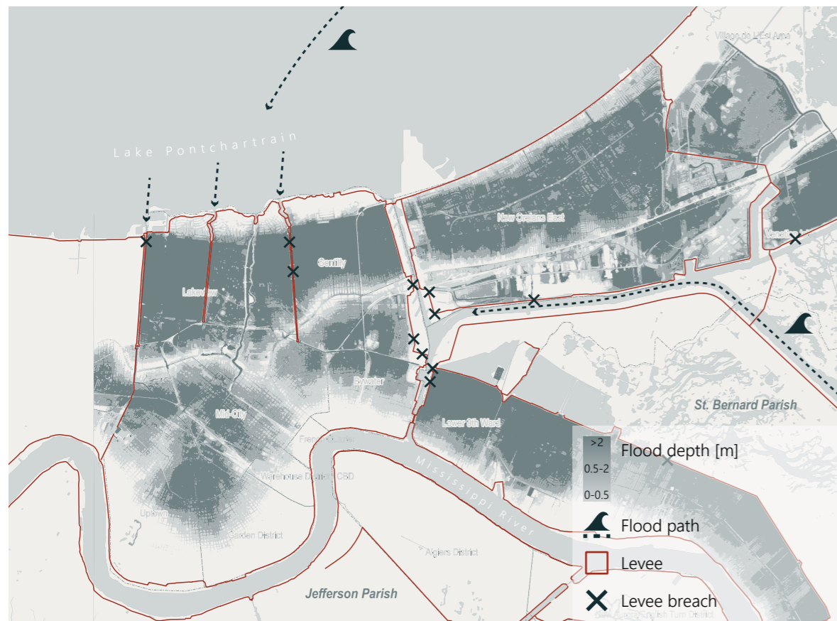
Figure 5 - Development of storm surge through the canals, levee breaches and extent of flooding (source: U.S. Department of Housing and Urban Development (2005), Marshall (2015), elaborated by author).
