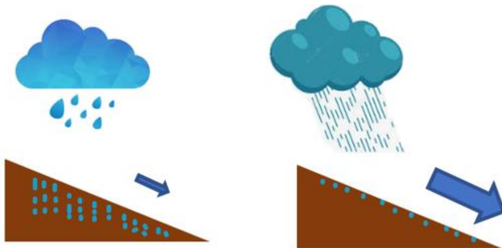
Figure 3.4.4: Low rainfall intensity results in large soil infiltration and small runoff (left); high rainfall intensity results in high runoff and less infiltration.
