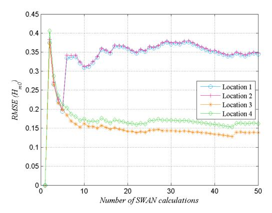
Figure 9 RMSE of  $H_{m0}$  as a function of the number of Monte Carlo samples with variation of model parameters.
