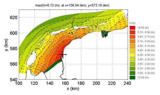
Figure 5 Variation of water level with scaled winds, obtained from Alkyon (2007c). The black cross indicates the location of the highest water level.
