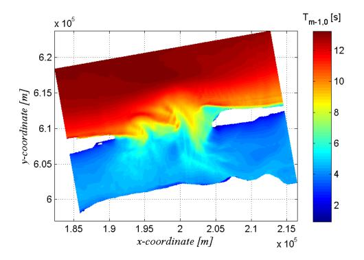
Figure 8  $T_{m-1,0}$  resulting from the reference calculation
