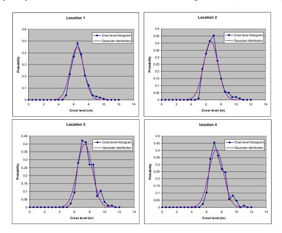
Figure 18 Probability density distributions of crest levels from the uncertainty analysis. Also shown are Gaussian distributions using the mean and standard deviation calculated from the sample set.
