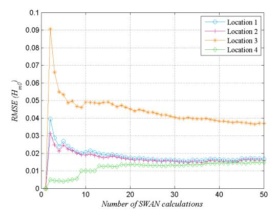
Figure 10 The RMSE of  $H_{m0}$  as a function of the number of Monte Carlo samples with variation of <u>SWAN</u> input.
