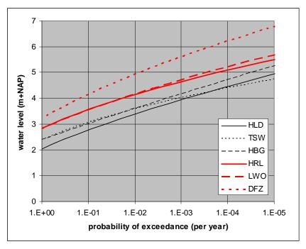
Figure 14 Probabilities of exceedance (POE) of water levels in the Wadden Sea (from WL 2007b). Locations are: HLD= Den Helder, TSW=Tereschelling, HBG=Huibertgat, HRL=Harlingen, LWO=Lauwersoog, DFZ=Delfzijl.
