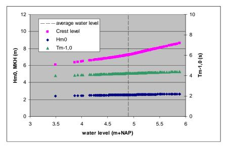
Figure 15 Correlation between samples of water level, wave conditions  $(H_{m0} \text{ and } T_{m-1,0})$  and critical crest level (CCL).
