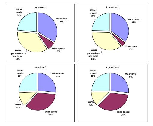
Figure 19: Relative contributions to the total uncertainty in critical crest level at the four locations under investigation. Locations 1 and 2 are next to shallow water, locations 3 and 4 are near a channel.
