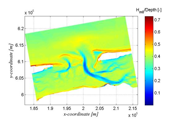
Figure 7 Relative wave height  $(H_{m0}/Depth)$  resulting from the reference calculation
