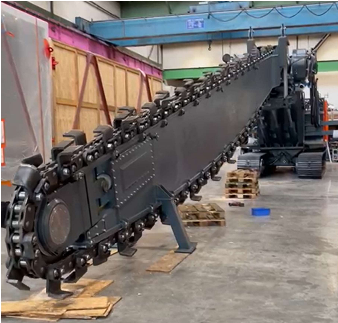
Figuur 1 Soilmix freesmachine (bron: HITEC Road & Partners)
