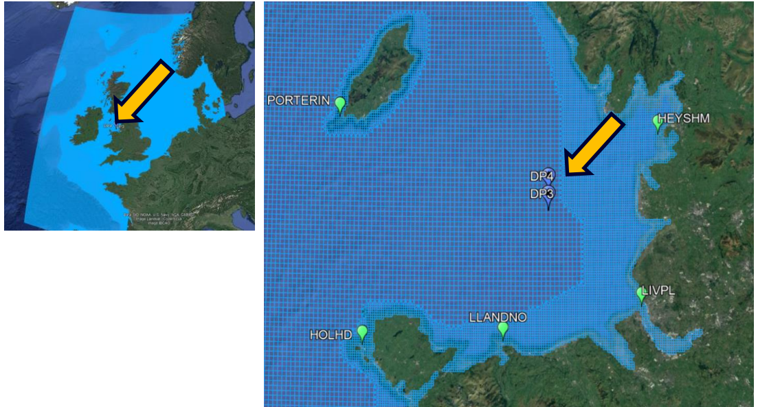
Figure 6.2 Computational grid (blue), locations DP3 and DP4 (blue markers), and tide gauge station (green markers) in the Morecambe Bay
