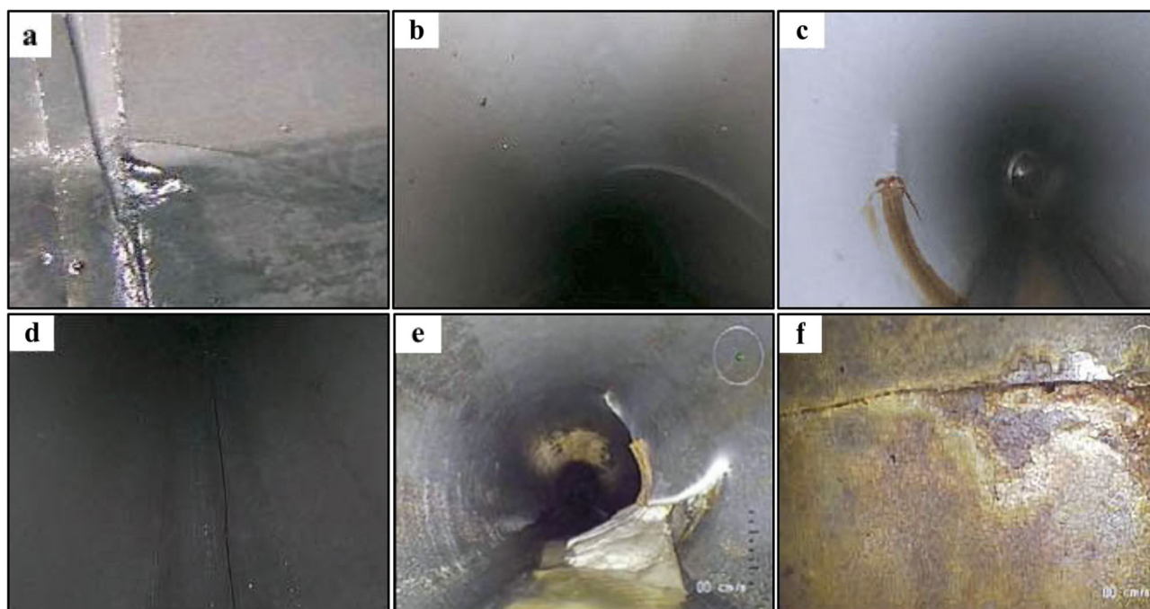
Figure 1. CCTV or Panoramio® footage of: (a) Exhumed pipe A-1 (DN 200, 43 years old) with crack at the connection. (b) Exhumed pipe A-2 (DN 200, 42 years old) with deformed top. (c) Exhumed pipe A-3 (DN 200, 41 years old) with pointy break at the side. (d) Exhumed pipe A-4 (DN 250, 39 years old) with crack at the bottom. (e) Exhumed pipe B-2 (DN 250, 39 years old) with break. (f) Exhumed pipe B-3 (DN 200, 23 years old) with complicated crack.
