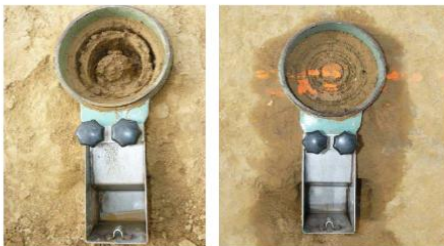
Figure 3.3. Appearance of the embankments after the external erosion tests: untreated embankments on the left and treated with lime on the right.
