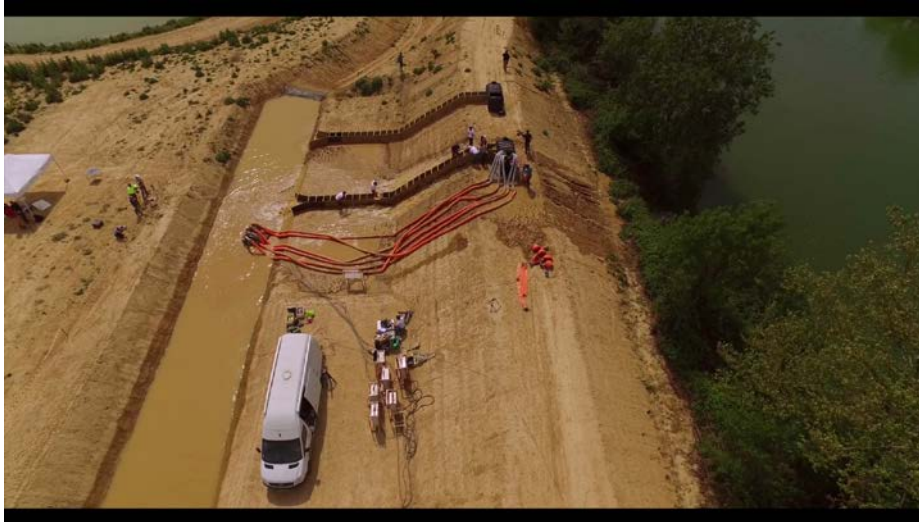
Figure 2. Overview of the site and overflow simulator. The Vidourle River is on the right.
