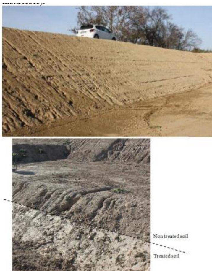
Figuur 3.1. ABOVE: Non – treated soil at left hand side, with erosion channels; lime treated soil at right hand side, with no erosion channel. BELOW: Contrast of external erosion resistance between non treated soil (upper part) and lime treated soil (lower part) (after Nerinx et al. 2016).
