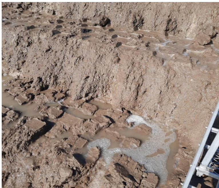
Figure 4-2 Footprint of the compacting machine (well compacted layer does not erode) and steep cliff in between (material erodes with increasing hydraulic load).
