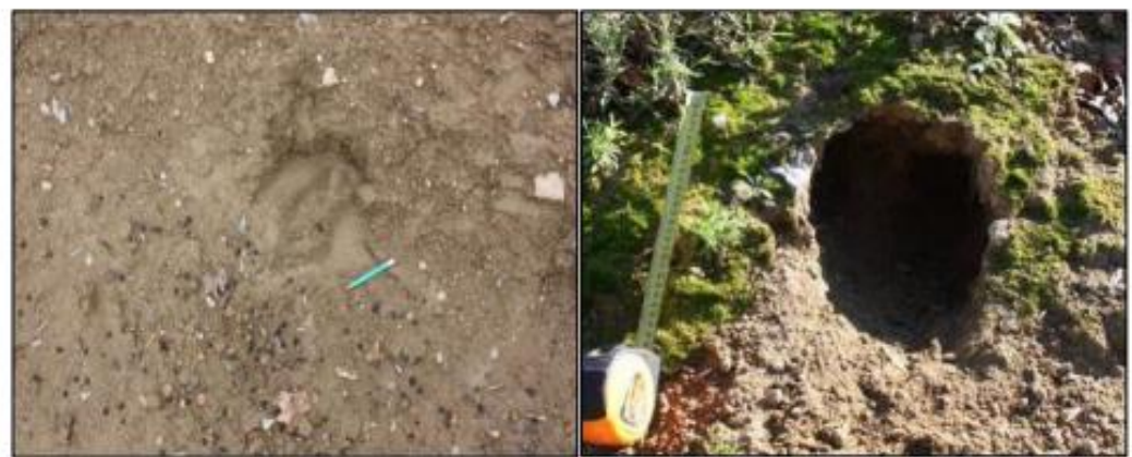
Fig. 6.11 Attempt to dig a burrow in a levee treated with 2.5% lime (left) and rabbit burrow dug in an untreated levee (right)
