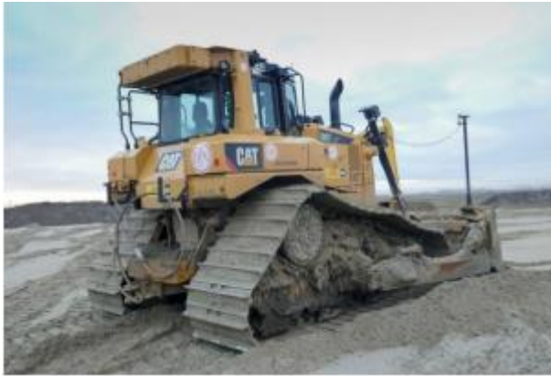
Figure 3-8 Machine for dozing and levelling (Figure courtesy Lhoist).
