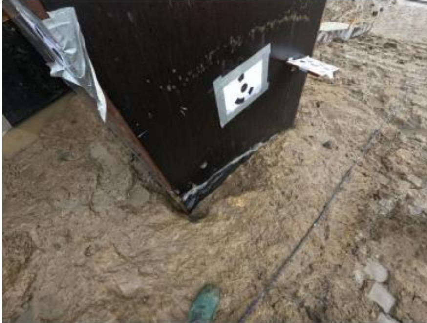
Figure 6-7 Erosion around the object after the final test (2m 50 lsm).
