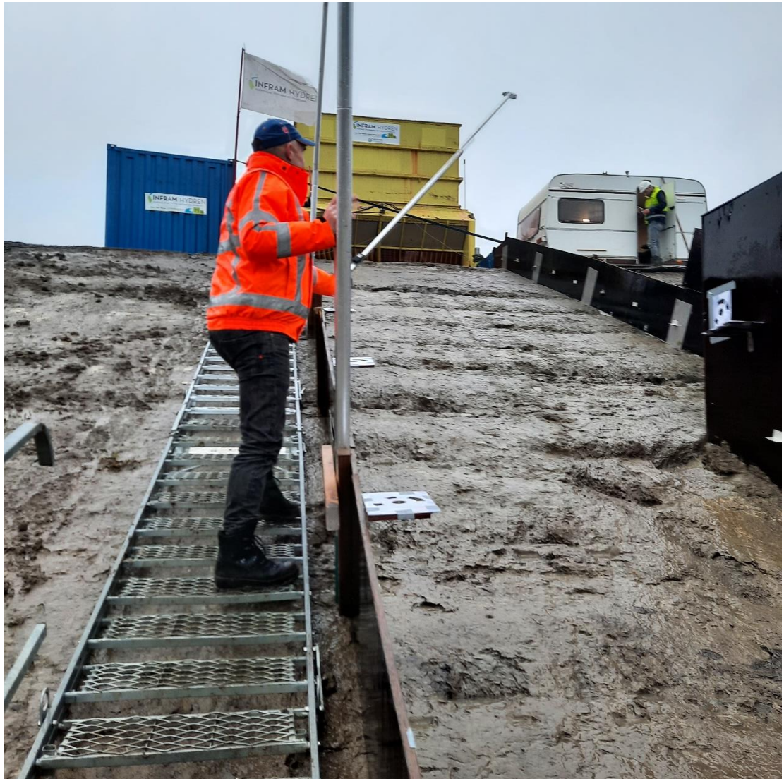
Figure 7-2 Measurement of the surface elevation using a GoPro camera mounted on a stick.
