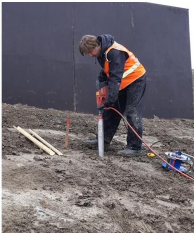
Figure 4-3 Use of drilling machine for taking samples in round B and C.
