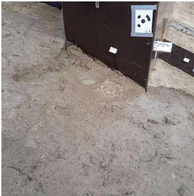
Figure 8-7 After the first tests: a maximum erosion depth of about 20 cm next to the obstacle.
