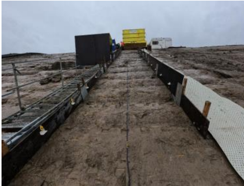
Figure 6-5 Test section 1B and erosion trench next to the obstacle after the test with 10 l/s/m'.
