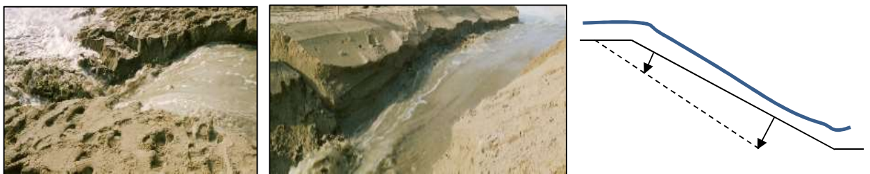
Figure 3: Surface erosion process during overflow (Visser, 1996)
