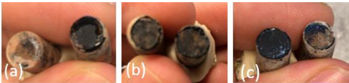
Figure 26 Failure mode for Granite aggregate: (a) adhesive (b) cohesive (c) mixed mode.
