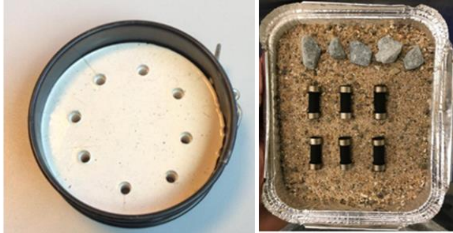
Figure 9 Preparation of mastic columns. Left picture: Silicon moulds used for sample preparation; right picture: samples resting in a sand bed during storage.
