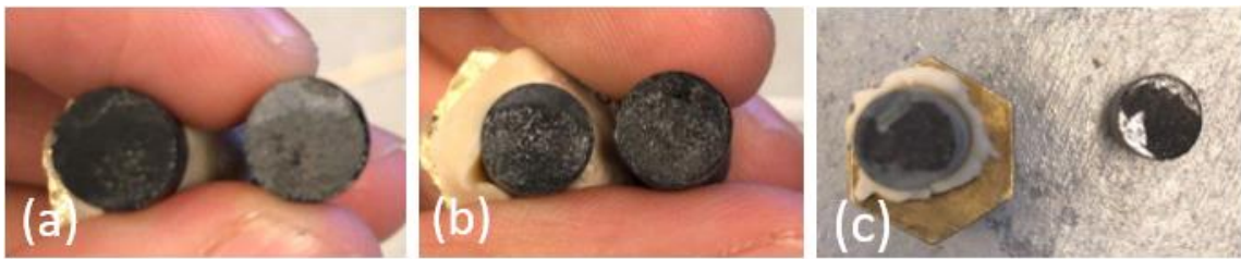
Figure 25 Failure mode for Bestone aggregates: (a) adhesive (b) cohesive (c) mixed mode.
