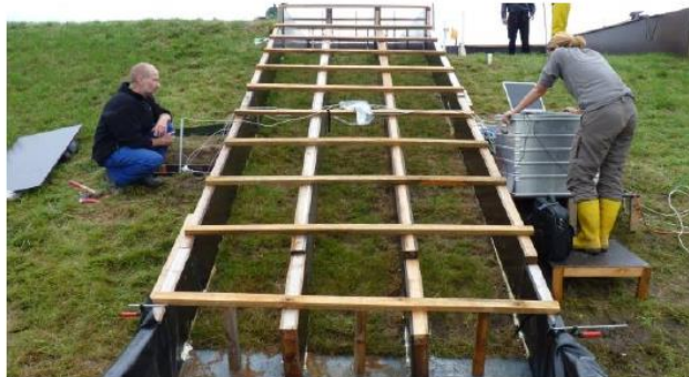
Figure All.12. Basic experimental set-up of the flume system
