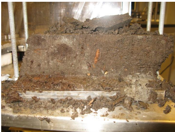
Figure 3.23 Test ID: DLDS -B1_Photos of the sample after shearing, during removal from the apparatus
