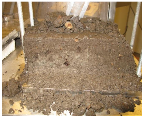
Figure 3.23 Test ID: DLDS -B1_Photos of the sample after shearing, during removal from the apparatus
