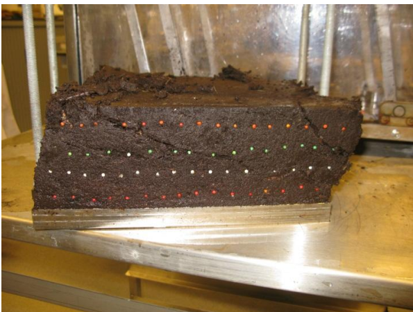
Figure 3.25 Test ID: DLDS -A3_Photos of the sample after shearing, during removal from the apparatus
