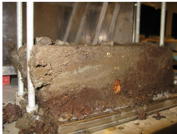
Figure 3.24 Test ID: DLDS -B2_Photos of the sample after shearing, during removal from the apparatus
