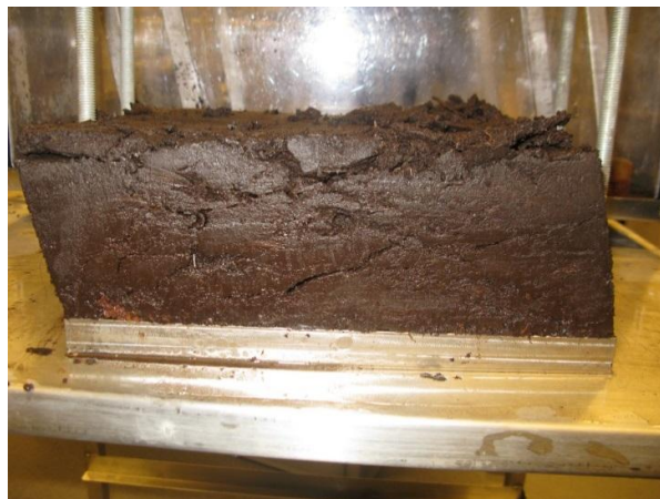
Figure 3.25 Test ID: DLDS -A3_Photos of the sample after shearing, during removal from the apparatus
