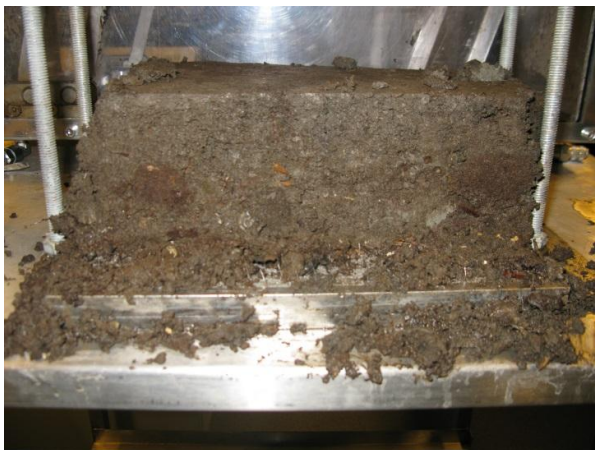
Figure 3.24 Test ID: DLDS -B2_Photos of the sample after shearing, during removal from the apparatus
