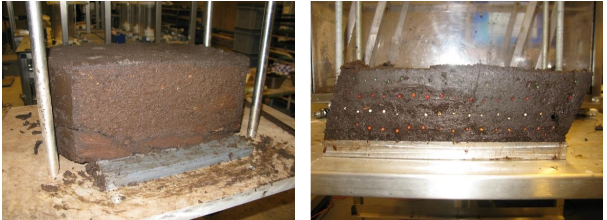
Figure 3.26 Test ID: DLDS -A4_Photos of the sample during trimming and after shearing, during removal from the apparatus
