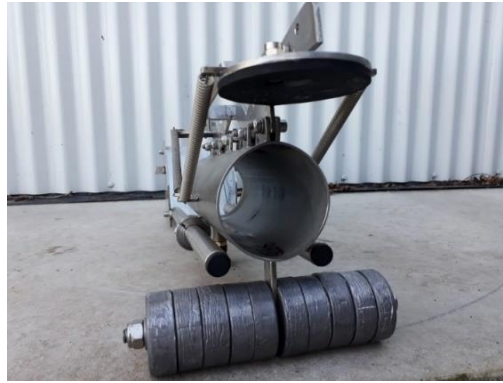
Figure 2.3.3 PIRANHA-instrument; In situ settling tube
