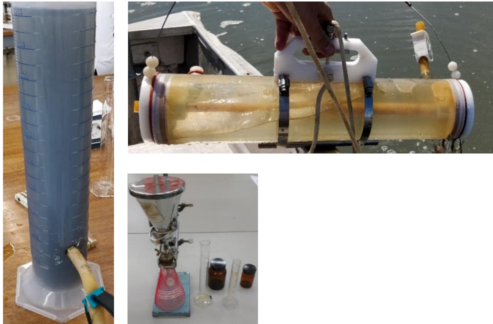
Figure 2.3.4 Laboratory settling tube with tap on side; water-sediment sampler; filtration set
