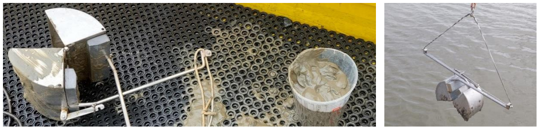
Figure 2.3.2 Mud sample taken with Van Veen-grab at location B
