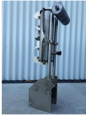
Figure 2.3.3 PIRANHA-instrument; In situ settling tube
