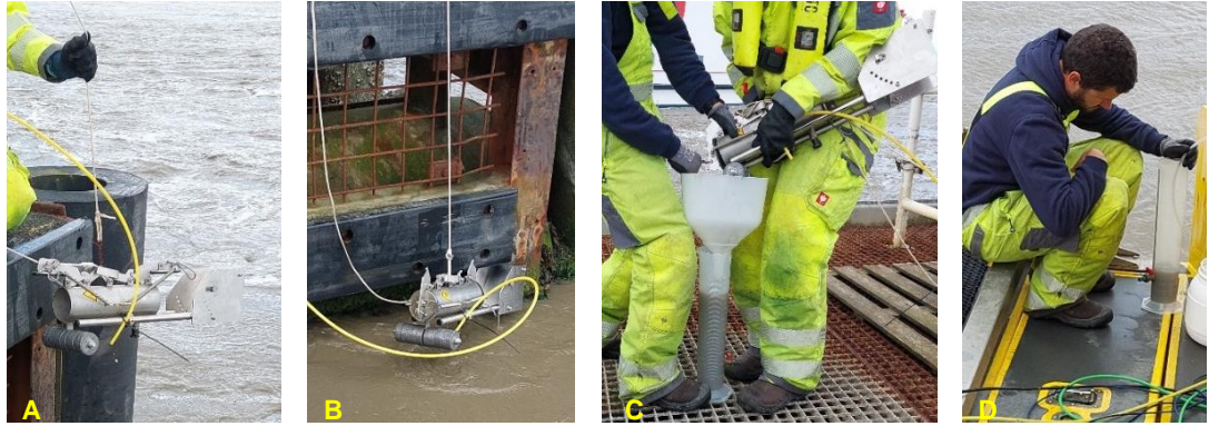
Figure 2.3.7 Piranha-instrument: A: lowered with open valves; B: raised with closed valves; C: samples transferred to settling tube; D: pump sample into settling tube
