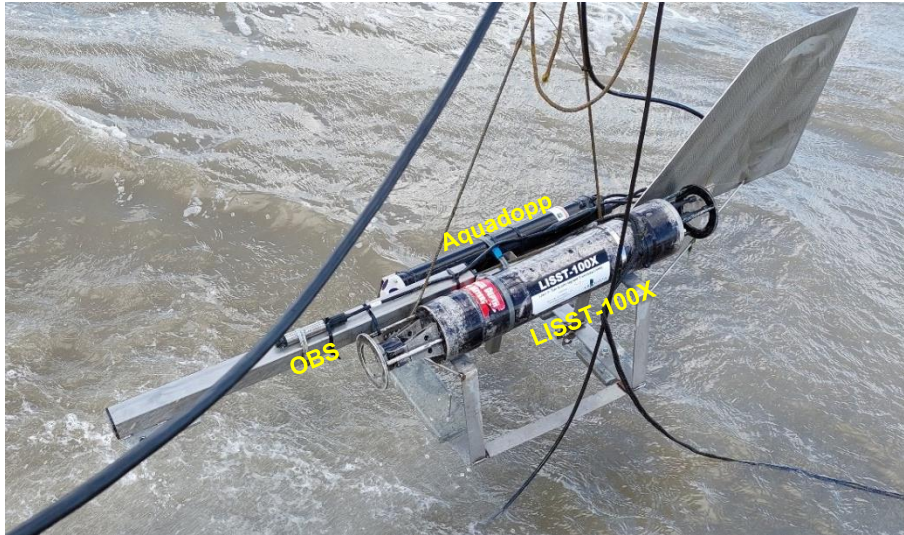
Figure 2.3.6 Bed frame (fish); Aquadopp for velocity; OBS for mud concentration; LISST-100X for particle size.
