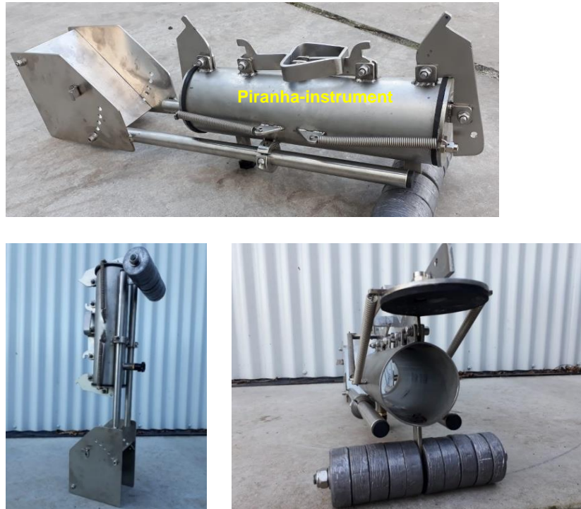
Figure 2.3.3 Piranha-instrument; In situ settling tube
