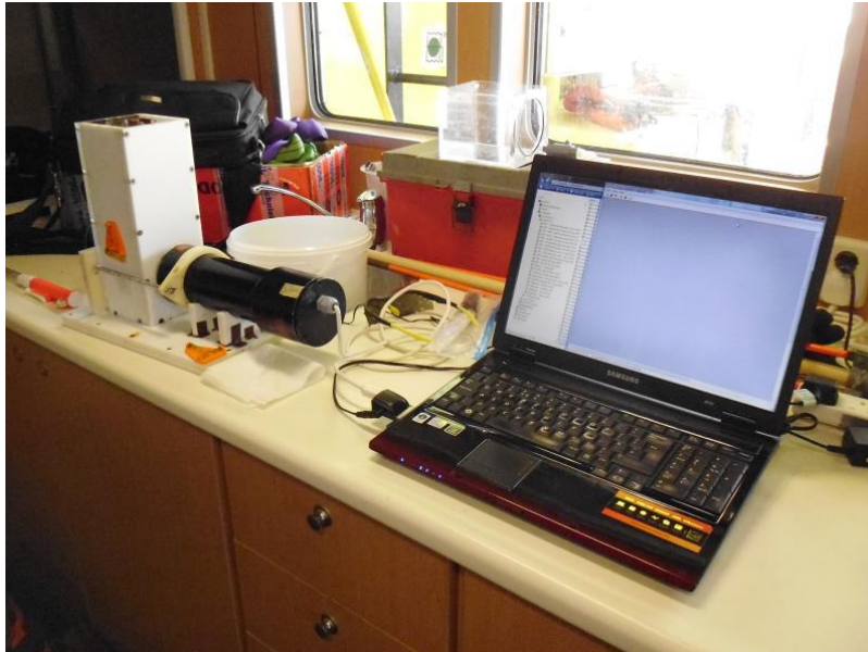
Figure 3.2.1 Laboratory setup of settling tube and video camera system (LABSFLOC-2-instrument)
