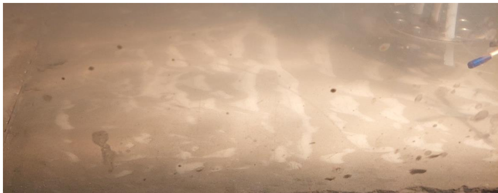
Figure C. 3: Bed with flat sand ripples/pots (light) and fines in troughs (grey/darker) during Test CC-2
