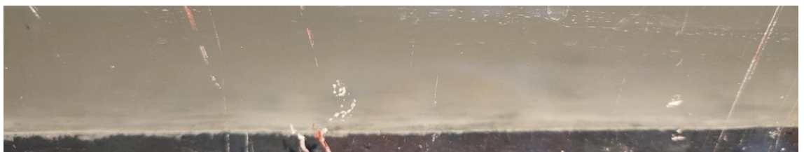
Figure Bed with ripples and sand transport (side view) during combined current+waves
