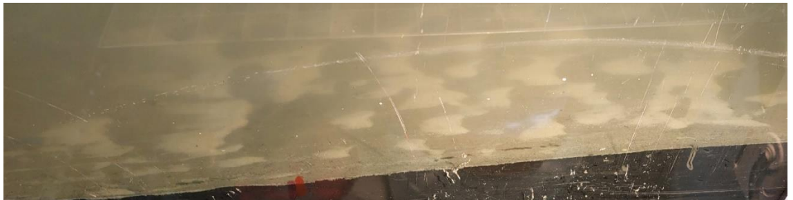
Figure Low, isolated bed ripples (side view) during waves alone H=0.08 m and H= 0.12 m
