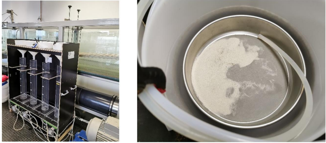
Figure 3.2.3 Sediment collection stack.
