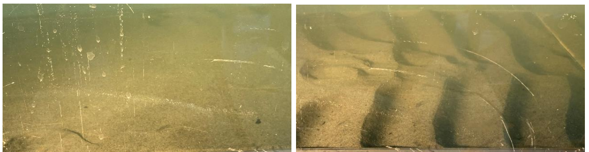
Figure B. 3: Initiation of ripples (left) and growing ripples (right) for Test BA-4 ( u_m=0.1 m/s).
