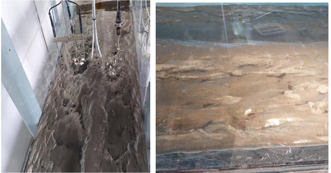
Figure Bed at end of tests; plan view (left) and side view (right); u_m=75 m/s, H=0.06 m
